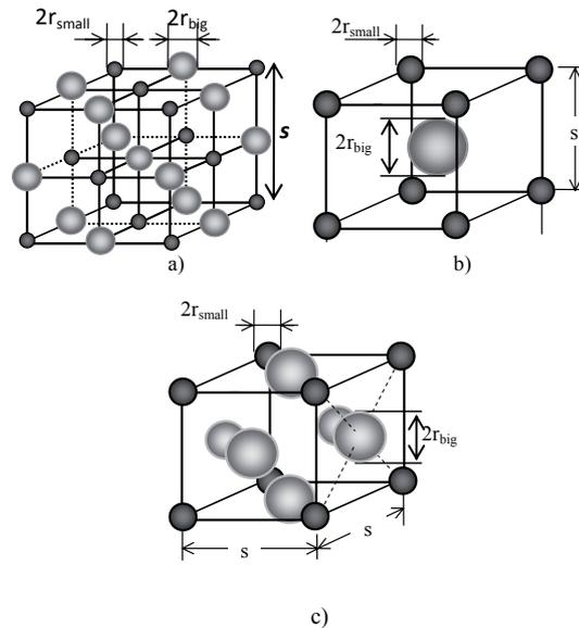
Fig. 1. a) Face centered NaCl cell; b) body-centered single cell; c) face-centered single cell.
