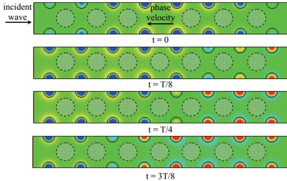
**Fig. 5.** Magnetic field patterns for four different moments of the period of time. The incident wave enters the structure from the left side, whereas the wave inside structure propagates from the right side to the left.
