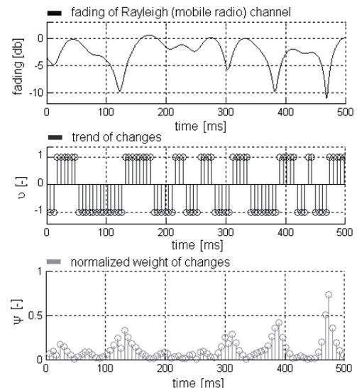
Fig. 3. Fading, trend and normalized weight of changes.
