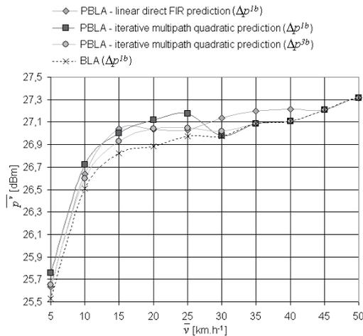
Fig. 8.  $\bar{p}^v$  of simulated PBLA and BLA algorithms.
