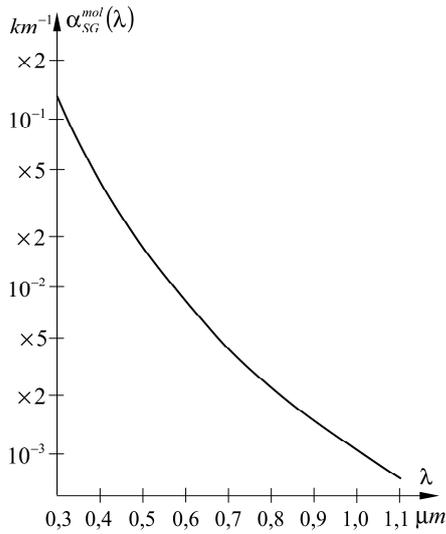
Fig. 3. Model representation of molecular extinction coefficient.
