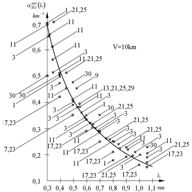
Fig. 1. Model representation of aerosol extinction coefficient when  $V = 10 \text{ km}$ .
