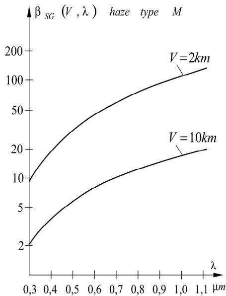
Fig. 4. Model relations  $\beta_{SG}(V=10 \text{ km}, \lambda)$  and  $\beta_{SG}(V=2 \text{ km}, \lambda)$  for an aerosol haze of the type M.
