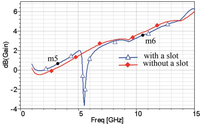
Fig. 9. Simulated gain of the antenna without and with a slot.
