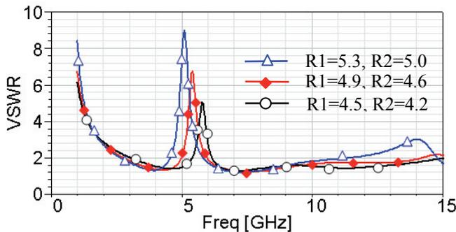
Fig. 6. Simulated VSWR for various  $R1$  and  $R2$  in mm with  $L12 = 6.7$  mm.
