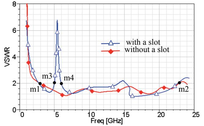
Fig. 2. Simulated VSWR of the antenna without and with a slot.
