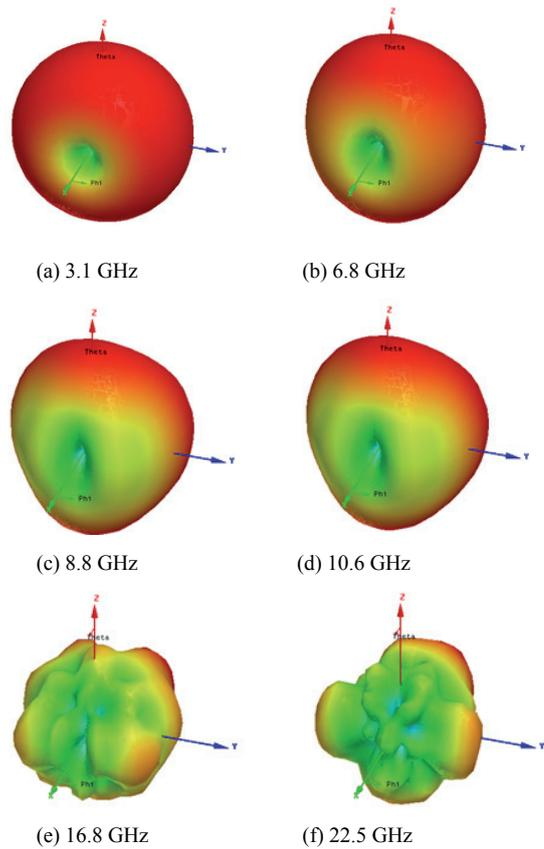
Fig. 7. Simulated radiation patterns at specific frequencies.
