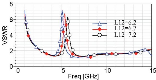
Fig. 5. Simulated VSWR for various  $L12$  in mm with  $R1 = 4.9$  mm and  $R2 = 4.6$  mm.
