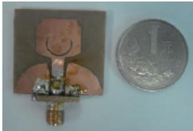
Fig. 10. Photograph of the fabricated antenna.
