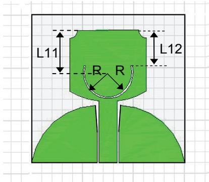
Fig. 4. Geometry of the antenna with a C-shaped slot,  $R1 = 4.9$  mm,  $R2 = 4.6$  mm,  $L11 = 8$  mm,  $L12 = 6.7$  mm.
