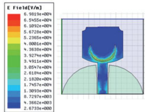
Fig. 8. Simulated current distribution of the antenna at 5.5 GHz.
