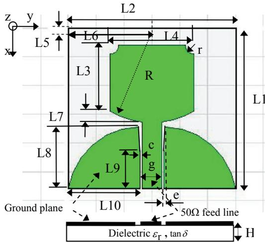
Fig. 1. Configuration of the proposed antenna.
