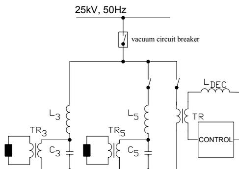
Fig. 1. FCE connection diagram.
