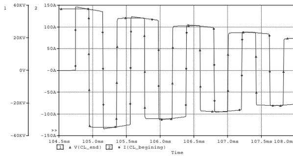
**Fig. 5.** The voltage waveform at the end of the contact line and the current waveform in the contact line after the short-circuit of the contact line at the feeding station.
