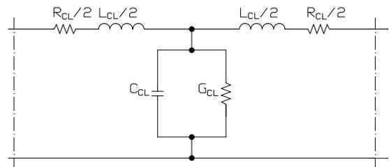
Fig. 3. Substitution diagram of the contact line.
