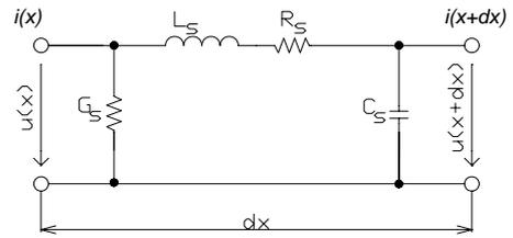
Fig. 2. Section of homogeneous line.
