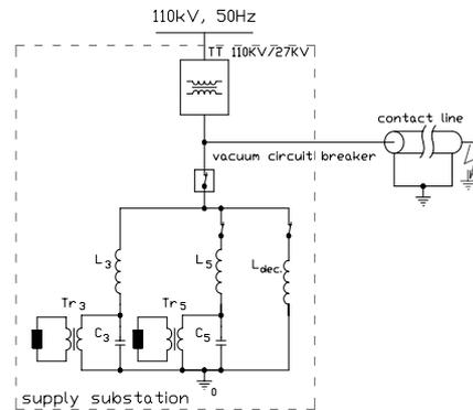
**Fig. 6.** Circuit diagram at short-circuit of the end of the contact line.
