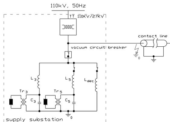
Fig. 4. Circuit diagram at short-circuit of the contact line at the feeding station.
