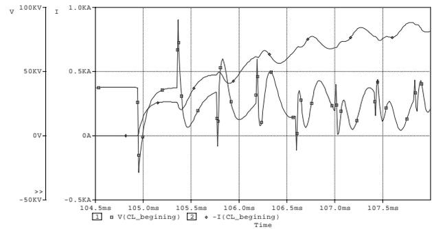
**Fig. 7.** The voltage waveform at the end of the contact line and the current waveform in the contact line after short-circuits on the contact line at the feeding station.
