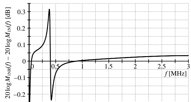
Fig. 10. The difference between the magnitude frequency responses of the SC biquad M_{1NR} and M_{1N} .
