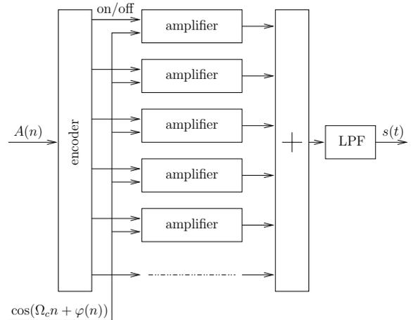
Fig. 7. Block diagram of the PSM transmitter.
