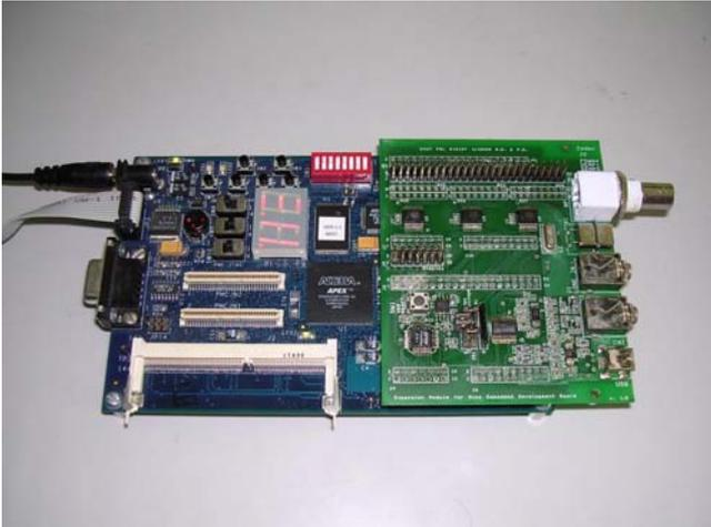
Fig. 8. FPGA development kit with the additional board.
