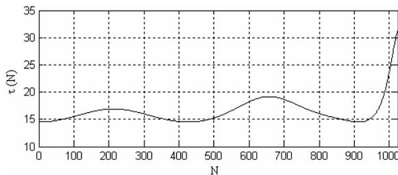
Fig. 5. The group delay of cascaded connection of the low-pass filter with the applied all-pass filter of the order 4.
