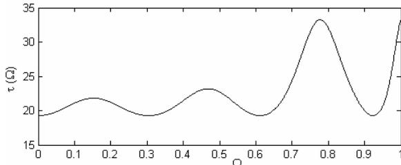
Fig. 4. The group delay of cascaded connection of the low-pass filter with the applied all-pass filter of the order 6.
