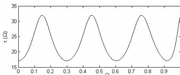
Fig. 10. The group delay of cascaded connection of the low-pass filter with the applied all-pass filter of the order 6.
