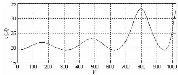
Fig. 7. The group delay of cascaded connection of the low-pass filter with the applied all-pass filter of the order 6.
