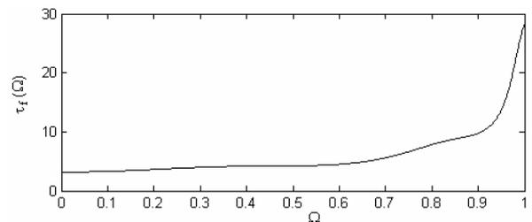
Fig. 1. The group delay of the low-pass filter.
