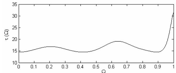
Fig. 2. The group delay of cascaded connection of the low-pass filter with the applied all-pass filter of the order 4.
