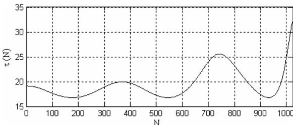
Fig. 6. The group delay of cascaded connection of the low-pass filter with the applied all-pass filter of the order 5.
