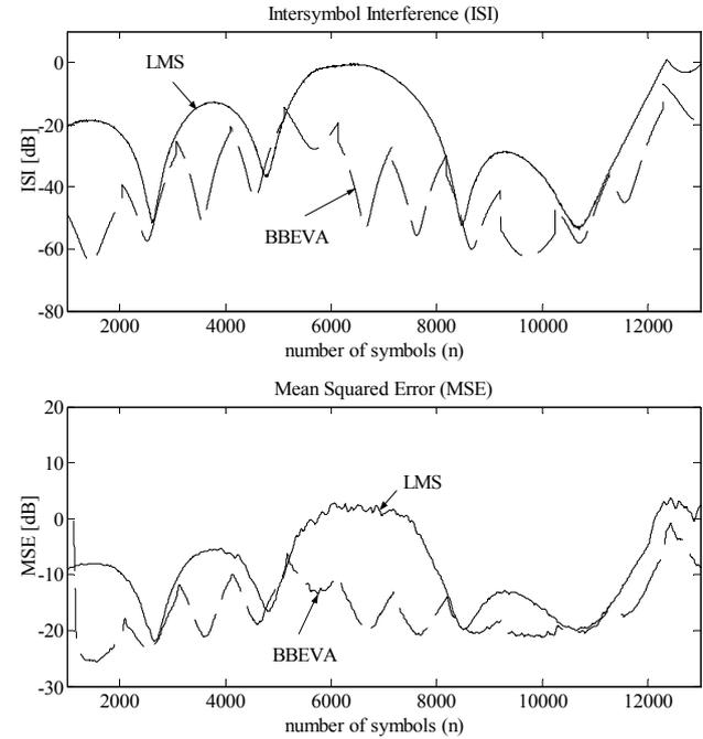
Fig. 3. The residual ISI (top) and MSE (bottom) for BBEVA and LMS algorithms.
