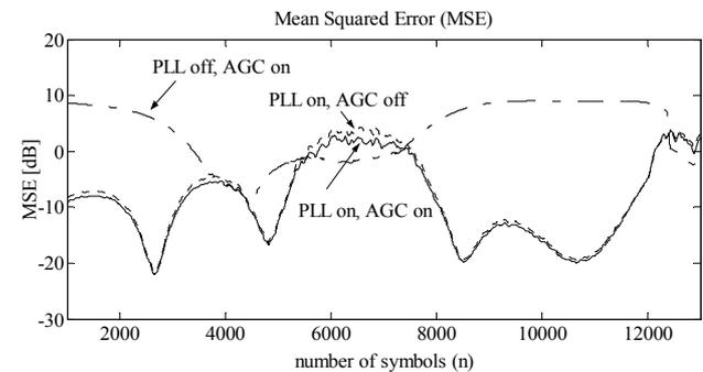
Fig. 5. The MSE for the LMS algorithm for different configurations.
