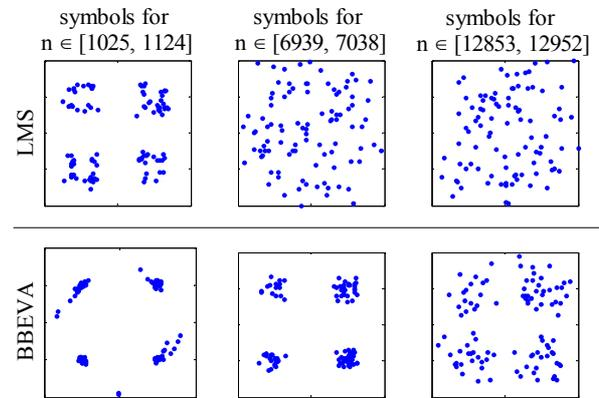
Fig. 4. Constellation of the equalized signal for LMS and BBEVA algorithms at different time (sample) instances.
