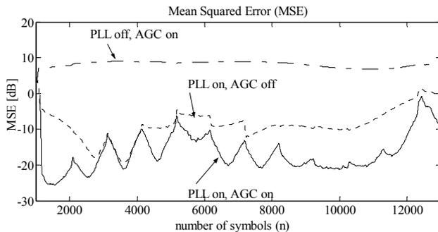
Fig. 6. The MSE for the BBEVA algorithm for different configurations.
