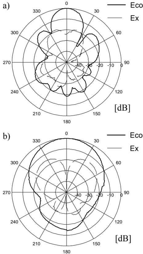
Fig. 5. Measured radiation patterns of CoMPA operating with  $TM_{05}$  mode in a) E-plane, b) H-plane.
