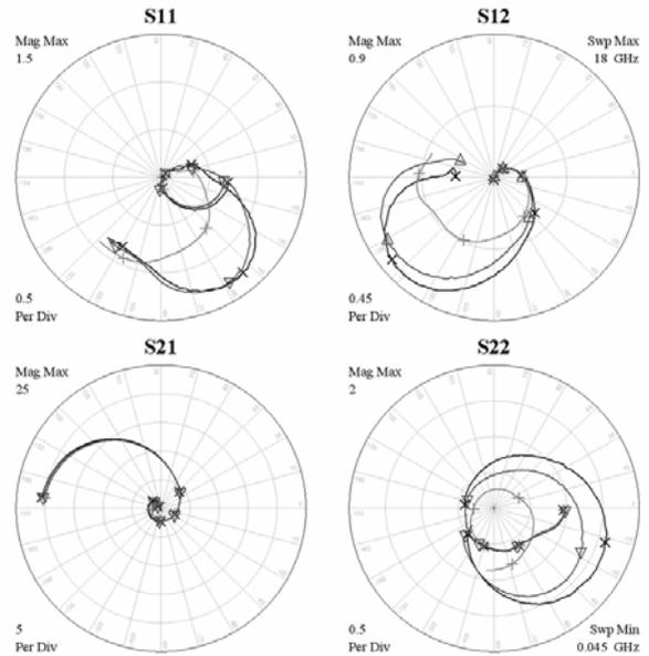
**Fig. 13.** S-parameters for assembly change in length of emitter feedback microstrip line from 0 mm to 1 mm at bias point 2V/10mA ( $\nabla$  measurement, + standard method,  $\times$  Mixed-mode method).
