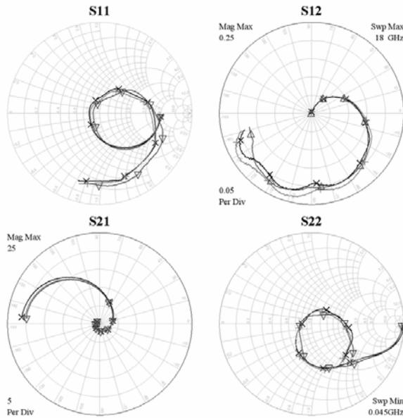
**Fig. 10.** S-parameters for assembly change in substrate parameters at bias point 1V/10mA ( $\nabla$  measurement on CuClad 233, + standard method transformation,  $\times$  Mixed-mode method transformation).
