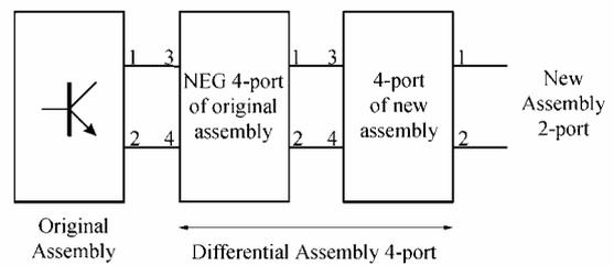
Fig. 6. Procedure of the Mixed-Mode correction method.
