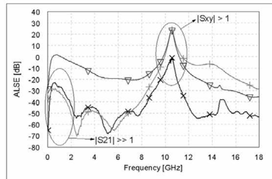
**Fig. 14.** Average least square error for assembly change in length of emitter feedback microstrip line from 0 mm to 2 mm at bias point 1V/10mA ( $\nabla$  comparison of measurements, + standard method transform,  $\times$  Mixed-mode method transform).
