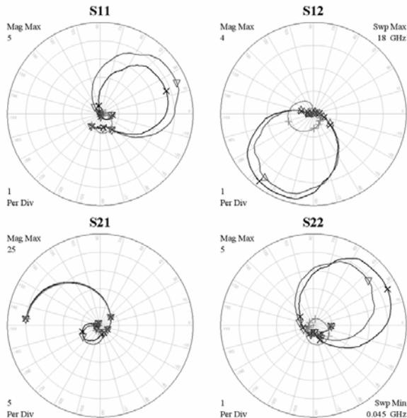
**Fig. 15.** S-parameters for assembly change in length of emitter feedback microstrip line from 0 mm to 2 mm at bias point 1V/10mA (V measurement for 2 mm microstrip, + standard method transform, × Mixed-mode method transform).
