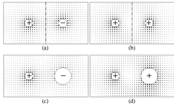
Fig. 4. Distribution of electric field at cross-section of a differential circuit. (a) Differential symmetrical mode - 2  $\times$  odd mode. (b) Common symmetrical mode - 1/2 even mode. (c) Differential asymmetrical mode. (d) Common asymmetrical mode.
