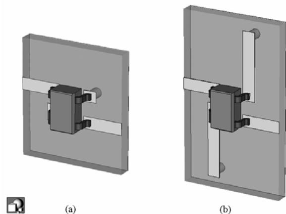
Fig. 1. Packaged SMD transistor. (a) Common emitter assembly. (b) Assembly with emitter feedback microstrip lines.
