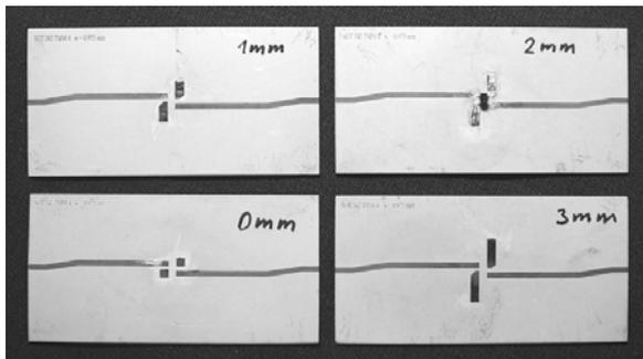
**Fig. 11.** Set of DUT samples with different lengths of the feedback microstrip line between emitter and via hole (substrate Rogers TMM4).
