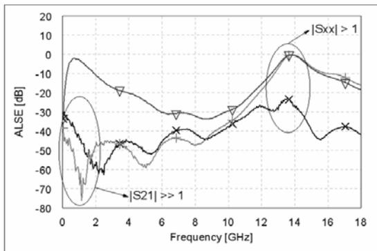
**Fig. 12.** Average least square error for assembly change in length of emitter feedback microstrip line from 0 mm to 1 mm at bias point 2V/10mA ( $\nabla$  comparison of measurements, + standard method transformation,  $\times$  Mixed-mode method transformation).
