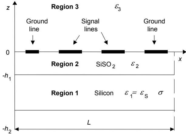
Fig. 1 Cross-sectioned view of the coplanar interconnect lines on lossy silicon substrate
