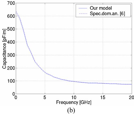
**Fig. 3** The frequency response of (a) conductance per unit length and (b) capacitance per unit length. The solid lines in the figures are obtained with our model, and the dashed lines are the result from the spectral domain approach.
