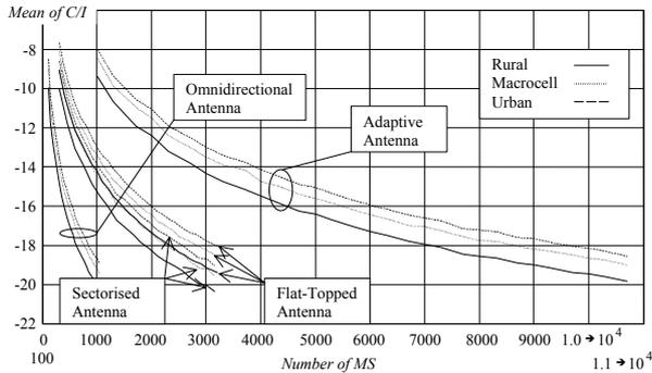
**Fig. 3** Mean value of  $C/I$  vs. number of MS in the system – perfect power control
