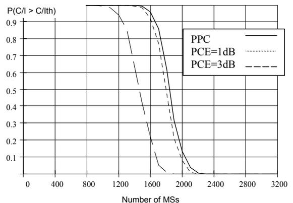
**Fig. 8** Probability  $P(C/I > C/I_{th})$  vs. number of MSs (rural environment, flat-topped antenna)
