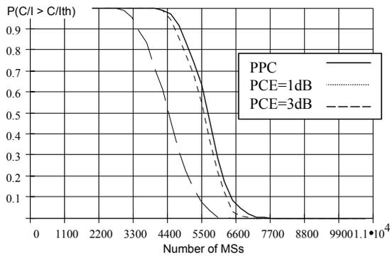
Fig. 9 Probability  $P(C/I > C/I_{th})$  vs. number of MSs (rural environment, adaptive antenna)
