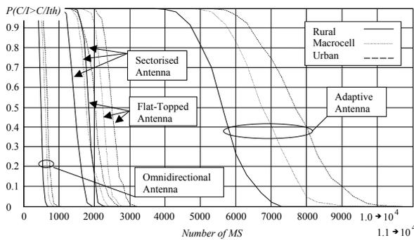
**Fig. 4** Probability  $P(C/I > C/I_{th})$  vs. number of MS in the system – perfect power control
