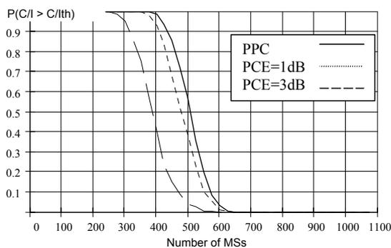
**Fig. 5** Probability  $P(C/I > C/I_{th})$  vs. number of MSs (rural environment, omnidirectional antenna)
