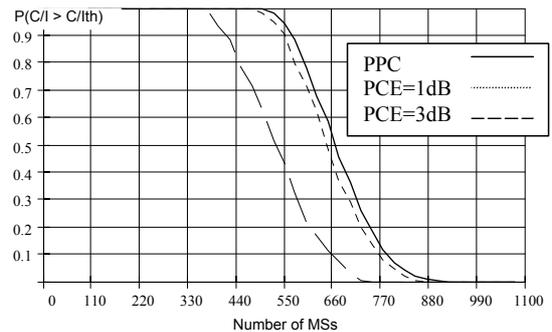
**Fig. 6** Probability  $P(C/I > C/I_{th})$  vs. number of MSs (urban environment, omnidirectional antenna)
