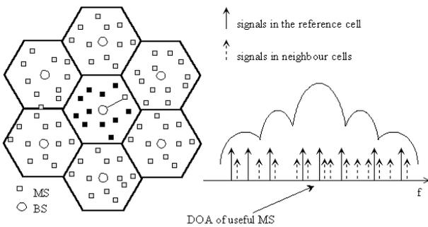
Fig. 1 Radiation pattern adaptation for CDMA system
