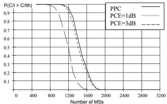
**Fig. 7** Probability  $P(C/I > C/I_{th})$  vs. number of MSs (rural environment, sectorized antenna)
