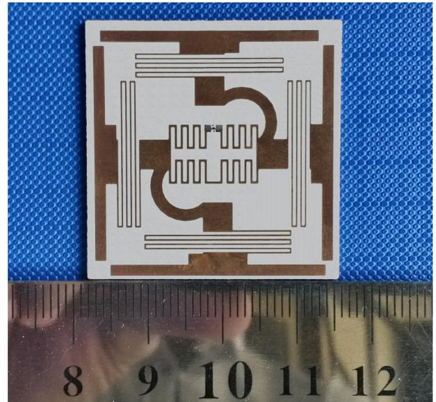
Fig. 4. Fabricated CP RFID tag antenna.
