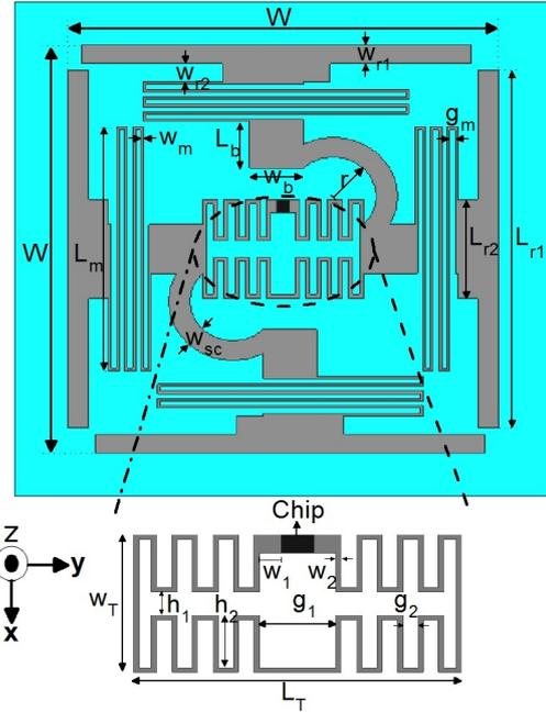
Fig. 1. Geometry of RFID CP tag antenna.
