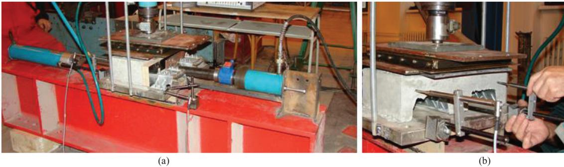
Fig. 1. (a) Small-scale shear test set-up; (b) concrete block movement measuring devices.
