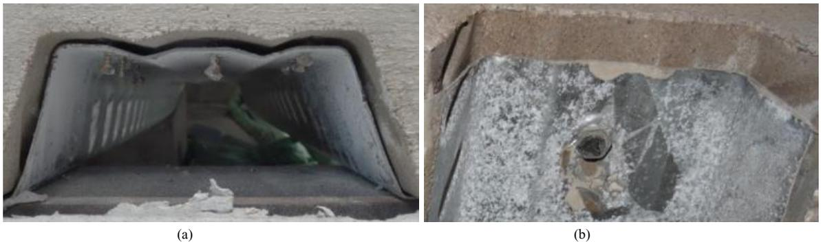
Fig. 4. (a) The failure mode of small diameter screws; (b) the failure mode of big diameter screws.
