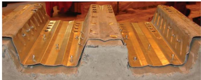
Fig. 2. (a) Comparison of shear resistances of the specimens with screws and without screws; (b) the specimen with screws after the test.
