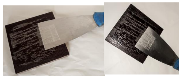
Figure 1. An easily-separable layer on the surface of the cladding
