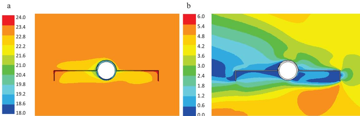
Fig. 2. ANSYS Fluent results – case E – (a) Static temperatures [°C]; (b) Velocity [m/s].
