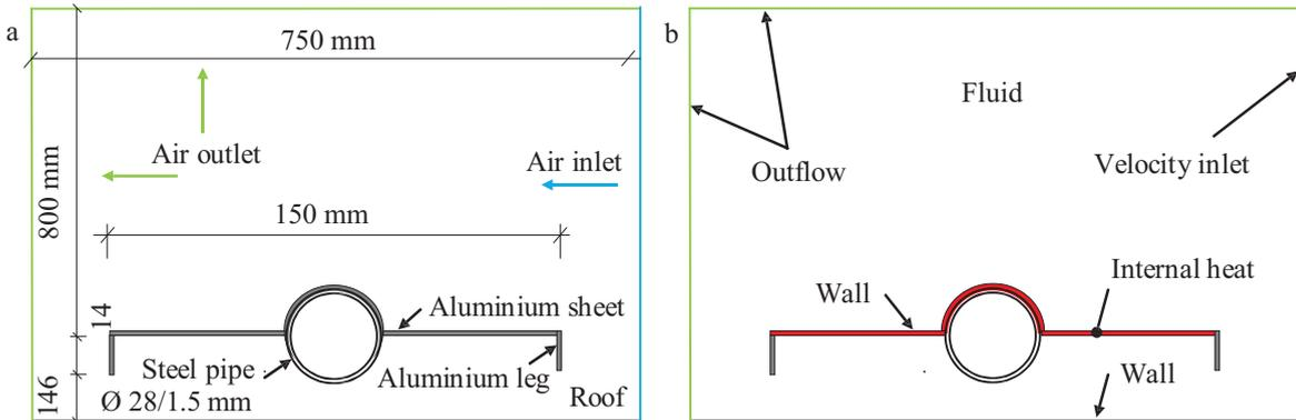
Fig. 1. (a) Geometry of the panel; (b) Boundary conditions used in ANSYS Fluent.
