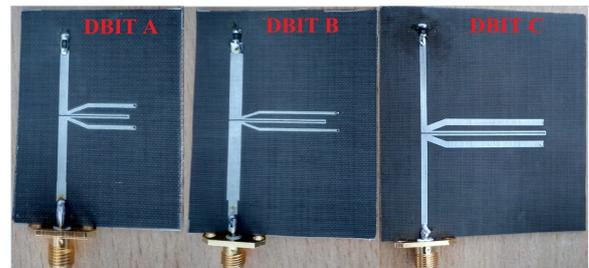
Fig. 7. Photograph of the fabricated prototypes with transforming ratios of 10, 20 and 30.
