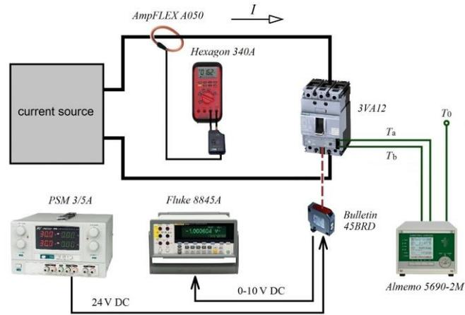
**Figure 2:** Measurement of thermostatic bimetal deflection
