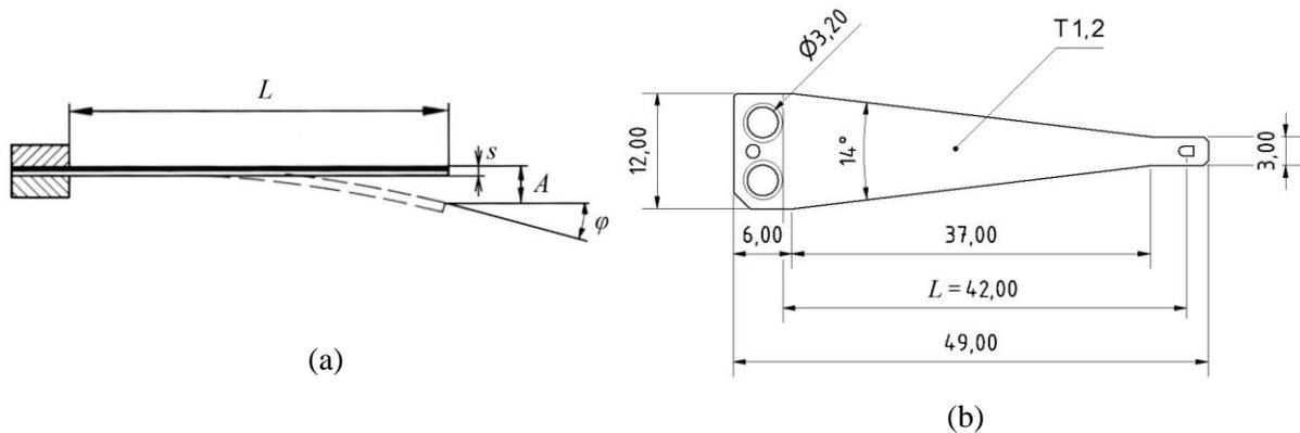
**Figure 1:** Deflection of straight thermostatic bimetal cantilever strip (a) and dimensions of the strip in trip unit (b)
