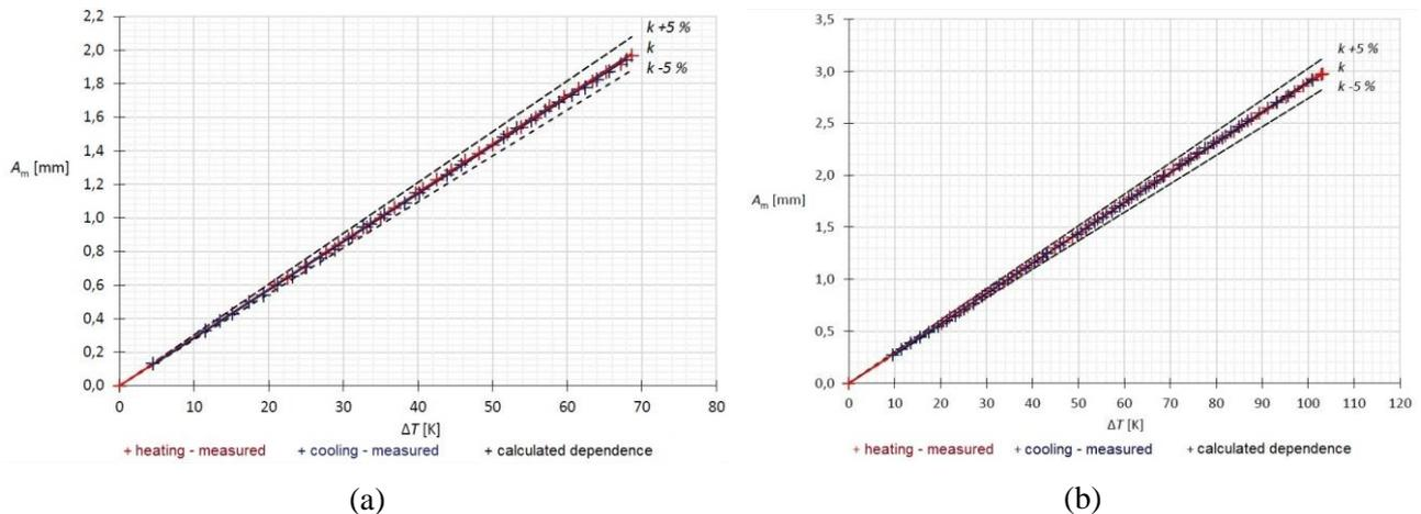
**Figure 3:** Measured bimetallic strip deflection depending on temperature change for heating by current of 262,5 A (a) and 325 A (b)
