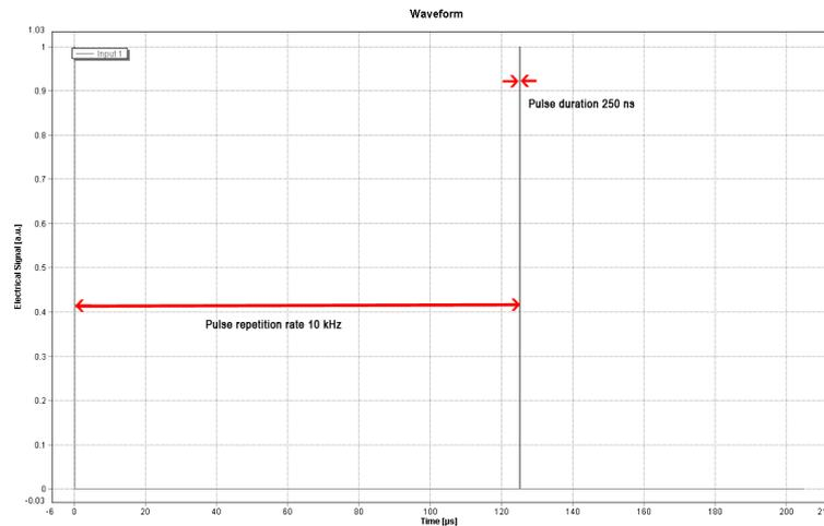
**Figure 2:** Signal with pulse duration of 250 ns and repetition rate of 10 kHz
