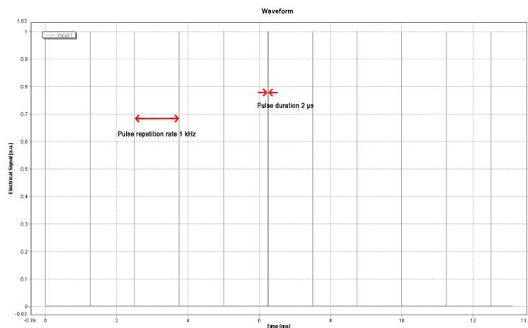
**Figure 3:** Signal with pulse duration of 2000 ns and repetition rate of 1 kHz
