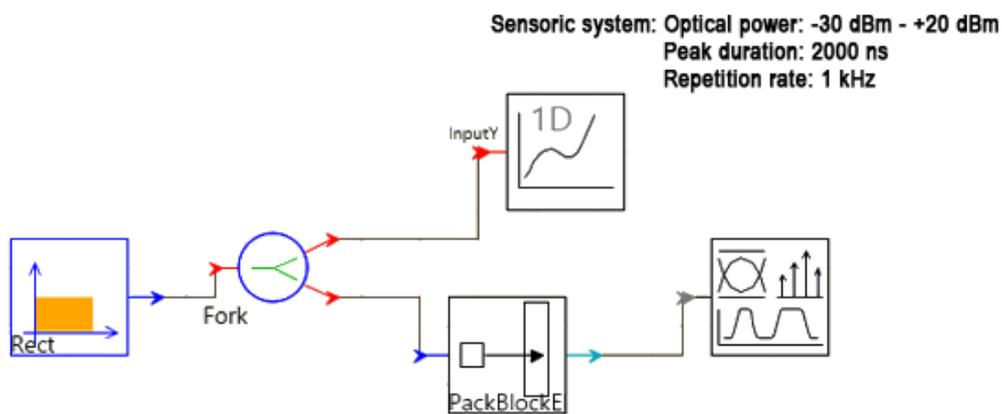
**Figure 1:** Simulation of pulse generator for  $\phi$ -OTDR.
