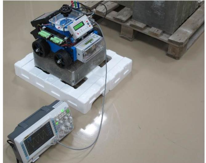
Fig.4. The compact NDT measurement and recording device to evaluate the impedance module/phase of the monitored component of the composite material sample. The apparatus operates as a semi-automatic monitoring system.
