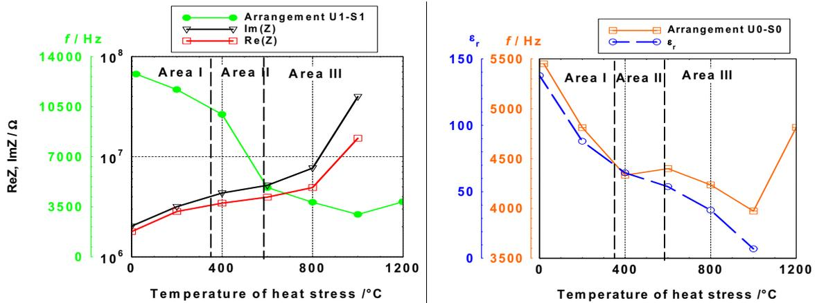
Fig. 3. (a) Discrete values of  $\text{Im}(Z)$ ,  $\text{Re}(Z)$  for 1kHz of electromagnetic field and dominant frequencies for impact echo method, for arrangement U1-S1(short way of wave); for different temperatures of annealing; (b) Values of dielectric permittivity versus frequency of electric field and dominant frequencies for impact echo method, for arrangement U0-S0(long way of wave), for different temperatures of annealing.
