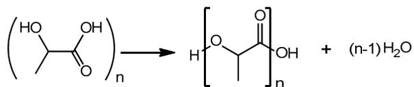
Figure 2. Scheme of autocatalytic lactic acid oligomerization.
