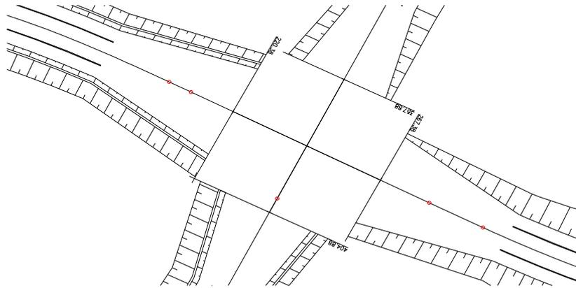
Figure 7.2 - Earthworks of road branches with bicycle extension
