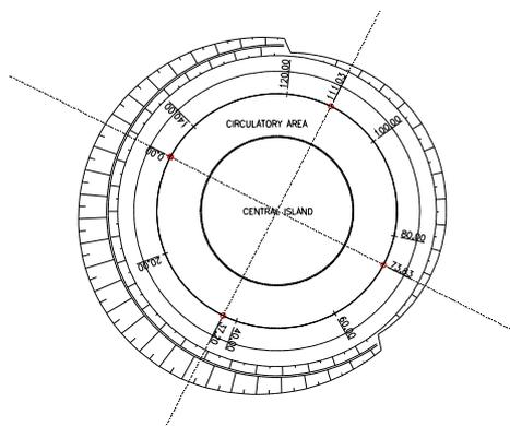
*Figure 7.1 - Earthworks of circulatory area with bicycle extension*
