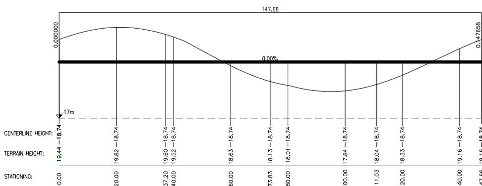
Figure 5.2 - Vertical alignment
