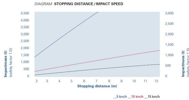
FIGURE 5. RAWIE 16 ZEB, stopping distance/impact speed/impact mass diagram, safety coefficient 1,0 and 1,5 [9]
