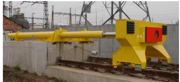
FIGURE 1. Example of hydraulic buffer stop (Oleo comp.) [7]
