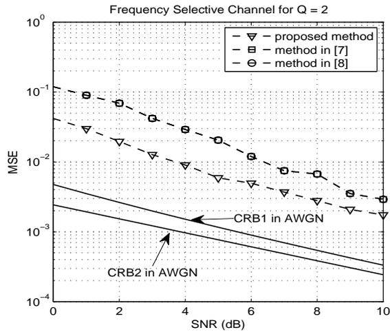
Fig. 6. Estimation performance in frequency selective channel for  $Q = 2$ .
