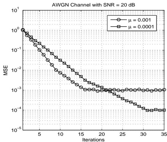
Fig. 8. Convergence performance in AWGN channel with SNR = 20 dB for  $Q = 4$ .
