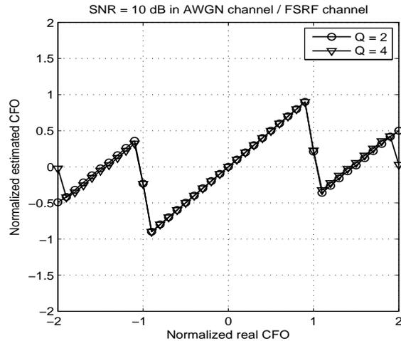
Fig. 3. Estimation range in AWGN channel for  $Q = 2, 4$ .
