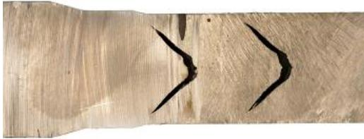
Fig. 1.2: Central bursting initiation during forward extrusion [1]
