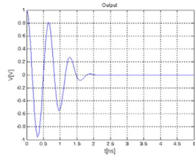
**Fig. 10.** Output signal of a pulse with  $f_0 = 1.5$  GHz and  $\tau_0 = 1$  ns and UWB radar reception with Hamming window.
