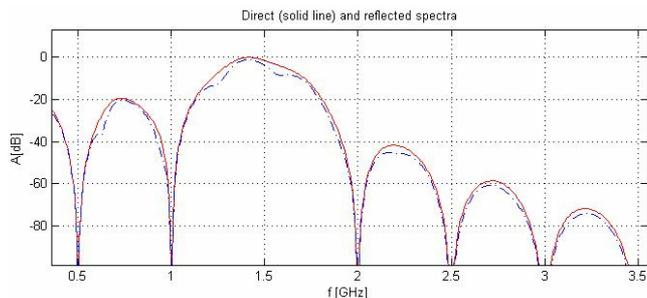
**Fig. 11.** Direct (solid line) and reflected spectra for a small transmitting antenna, heights  $h_1 = 1.5$  m and  $h_2 = 0.4$  m and distance  $r = 15$  m.
