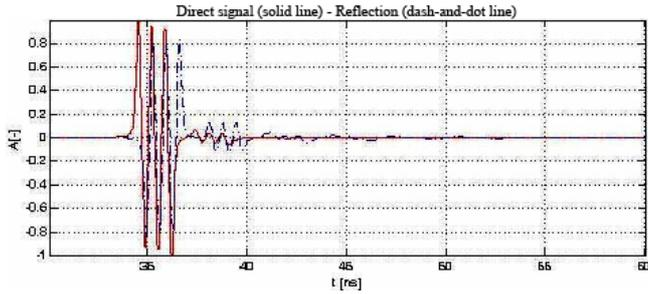
Fig. 4. Direct (solid line) and reflected (dot and dash line) signals for a small transmitting antenna,  $h_1 = 1.5$  m,  $h_2 = 0.4$  m and  $r = 10$  m.
