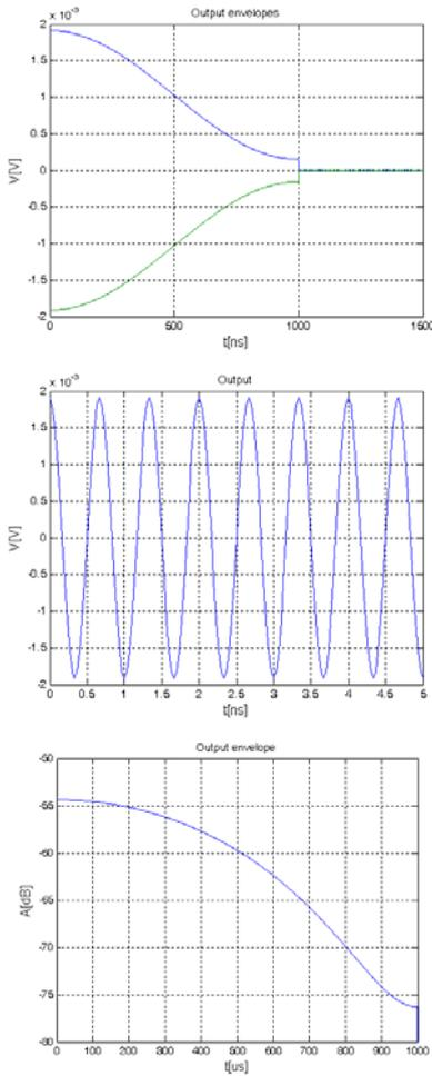
**Fig. 8.** Filter output signal of narrowband radar for pulse with  $f_0 = 1.5$  GHz and  $\tau_0 = 1$  ns. a) Envelope of output signal with linear scaling, b) Detailed view and c) Logarithmic scaling (dB) of output signal envelope
