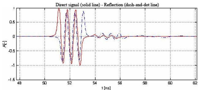
Fig. 5. Direct (solid line) and reflected (dot and dash line) signals for a small transmitting antenna,  $h_1 = 1.5$  m,  $h_2 = 0.4$  m and  $r = 15$  m.
