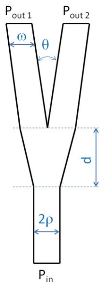
Fig. 2. Geometrical structure of the designed optical splitter.
