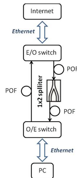
Fig. 12. Set up for testing transmission of the optical signal.
