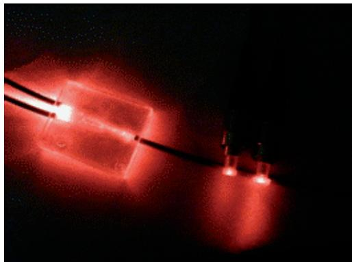
Fig. 10. Image of the 1x2 splitter transmitting the optical signal (650 nm).
