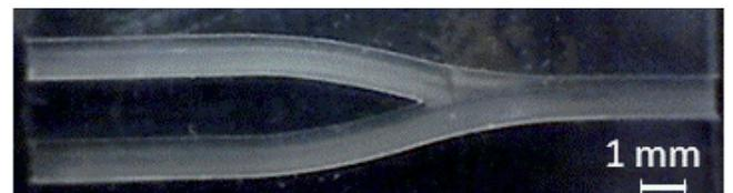
**Fig. 8.** Image of the 1x2 Y-groove substrate.
