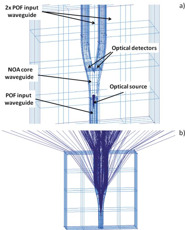
Fig. 4. a) Schematic view of the model of the designed splitters, b) view of the ray tracing diagram for 1x2 splitter.
