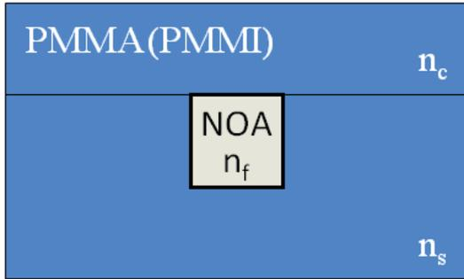
Fig. 1. Schematic view on the multimode optical waveguide cross-section ( $n_c = n_s$ ).
