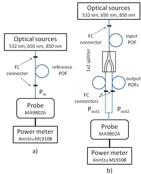
Fig. 11. Set up for insertion optical loss measurement.
