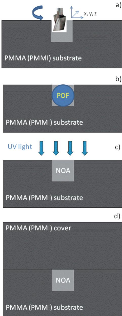
**Fig. 6.** Fabrication process of the optical splitters, a) CNC machining into polymer substrate, b) inserting of standard POF waveguide, c) filling up taper region with core layer and applying UV curing process, d) assembling top cover layer.
