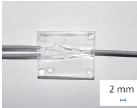
Fig. 9. Image of the 1x2 splitter fabricated from PMMA/NOA73 polymers with POF input/output waveguide.
