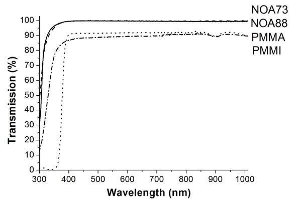
**Fig. 7.** Transmission spectra of waveguide core NOA73, NOA88 polymer and PMMA, PMMI substrates and cover layers.
