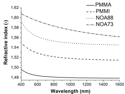
Fig. 3. Refractive indices of PMMA, PMMI, NOA polymers measured by ellipsometry.
