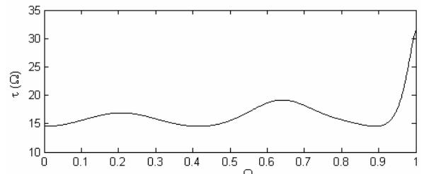
Fig. 2. The group delay of cascaded connection of the low-pass filter with the applied all-pass filter of the order 4.
