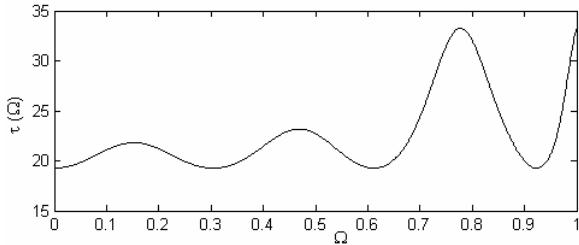
Fig. 4. The group delay of cascaded connection of the low-pass filter with the applied all-pass filter of the order 6.
