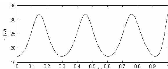
Fig. 10. The group delay of cascaded connection of the low-pass filter with the applied all-pass filter of the order 6.
