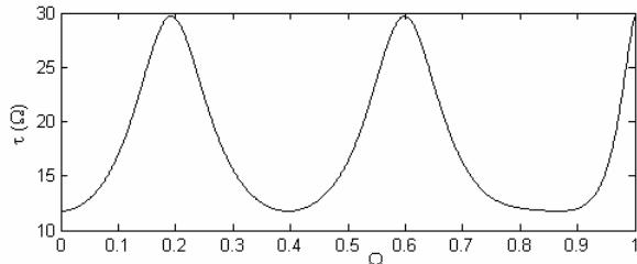
Fig. 8. The group delay of cascaded connection of the low-pass filter with the applied all-pass filter of the order 4.
