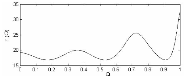
Fig. 3. The group delay of cascaded connection of the low-pass filter with the applied all-pass filter of the order 5.
