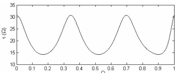
Fig. 9. The group delay of cascaded connection of the low-pass filter with the applied all-pass filter of the order 5.
