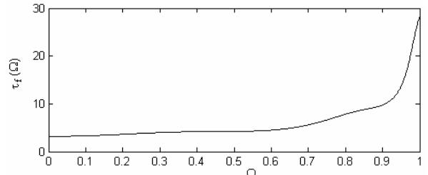
Fig. 1. The group delay of the low-pass filter.
