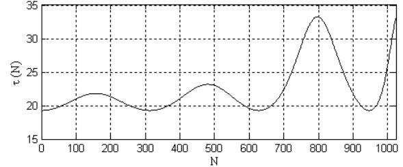
Fig. 7. The group delay of cascaded connection of the low-pass filter with the applied all-pass filter of the order 6.
