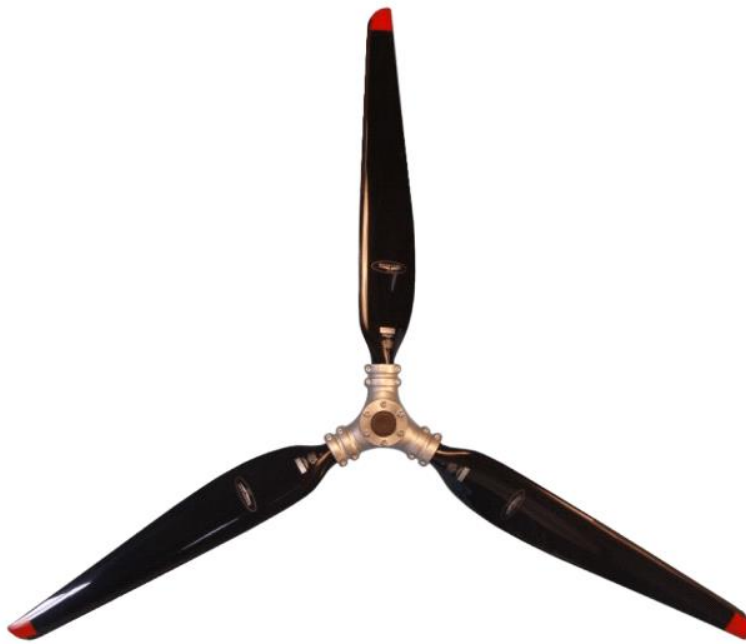
Picture 2. 2 proppeller : sensenich fixed 3- blade
