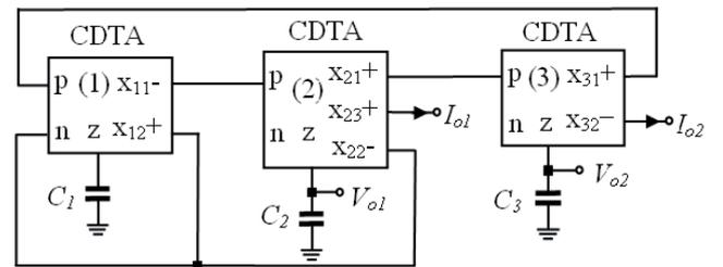
Fig. 3. The proposed current-mode quadrature oscillator.
