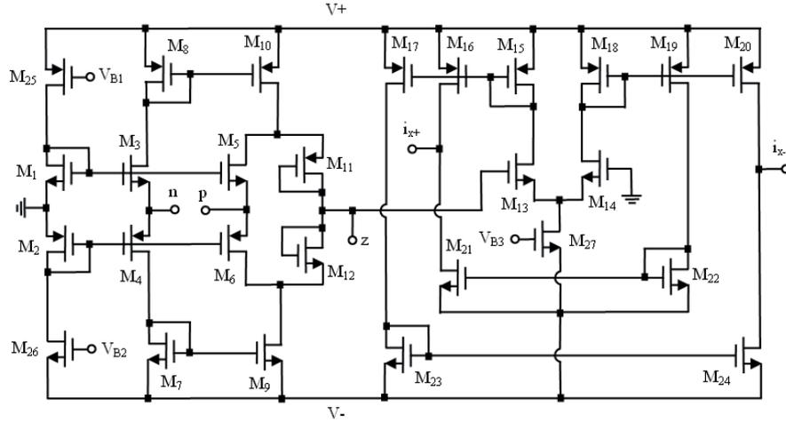
Fig. 2. CMOS-based CDTA.
