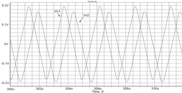
Fig. 5. The simulated voltage-mode quadrature output waveforms of Fig. 3.
