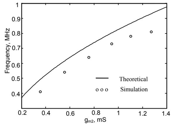
Fig. 6. Simulation result of the oscillation frequency of the circuit given in Fig. 3, which is obtained by varying the value of the transconductance  $g_{m2}$ .
