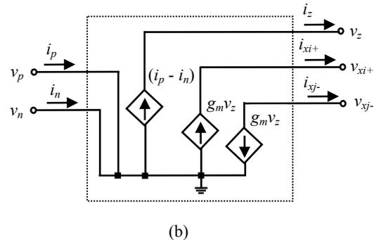
Fig. 1. (a) Circuit symbol of CDTA. (b) Equivalent circuit of CDTA.
