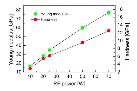
Figure 10: Young modulus and Hardness of pp-TVS layers depending on RF power
