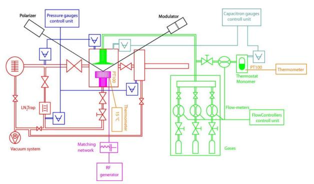
Figure 2: Schematic illustration of technological apparatus "A3" [23]
