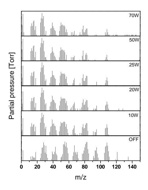
Figure 3: Comparison of mass spectra of plasma polymer layers deposited with different RF powers, in logarithmic scale
