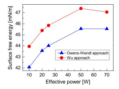
Figure 12: Dependence of surface free energy evaluated by Owens-Wendt and Wu approach on the magnitude of the input RF power
