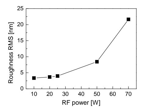
Figure 9: Dependence of the RMS roughness of the pp-layers from TVS on the RF power
