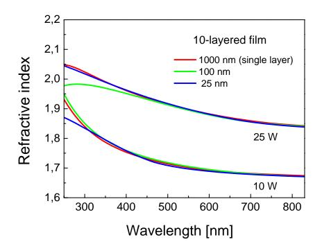
Figure 21: Dispersion curves for the refractive index of individual layers in 10-layered film. Dispersion curves corresponding to the individual layer of thickness 100 and 25 nm are compared with that for single layer film
