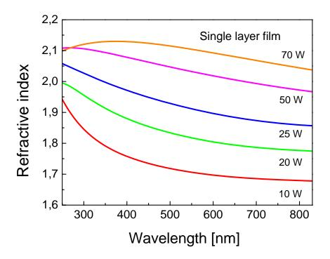
Figure 17: Dispersion curves for the refractive index of single layer film deposited at different RF powers
