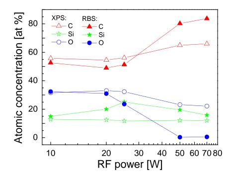
Figure 8: Comparison of atomic concentrations measured by XPS and RBS methods, depending on the RF power
