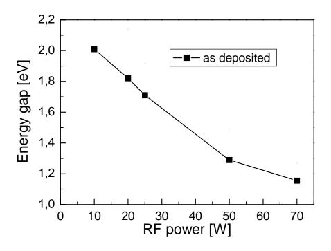
Figure 5: Dependence of the energy gap (eV) on the RF power (W) for set of single layer films measured after deposition
