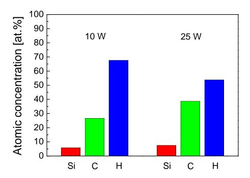
Figure 18: Elemental composition of single layer film deposited at an RF power of 10 W and 25 W
