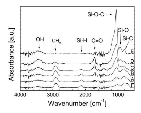
Figure 13: FTIR spectra of 0.5- $\mu$ m films irradiated by UV light (10 min – sample A; 33 min – B; 100 min – C; 333 min – D; 1000 min – E) compared with the reference sample (as-deposited, sample F)
