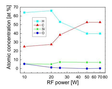
Figure 7: Dependence of the atomic concentration of pp-TVS layers on the RF power measured by RBS and ERDA
