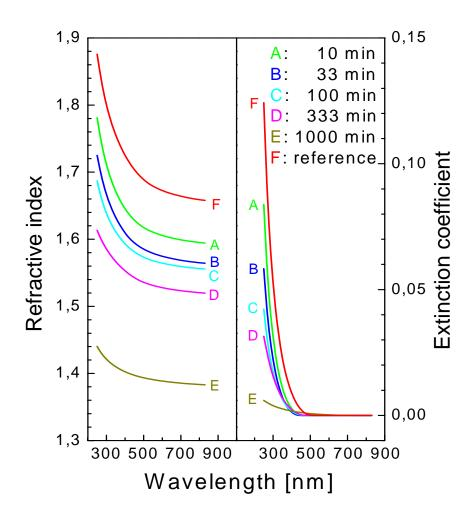
Figure 15: Dispersion curves of the refractive index and extinction coefficient for the reference (as-deposited film) and UV-irradiated samples.
