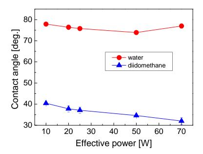
Figure 11: Dependence of the contact angle of all testing liquids on the magnitude of the input RF power
