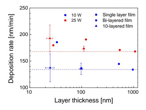
Figure 23: Deposition rate as a function of layer thickness. Dashed line corresponding to the deposition rate of single layer film is used as a guide for eye
