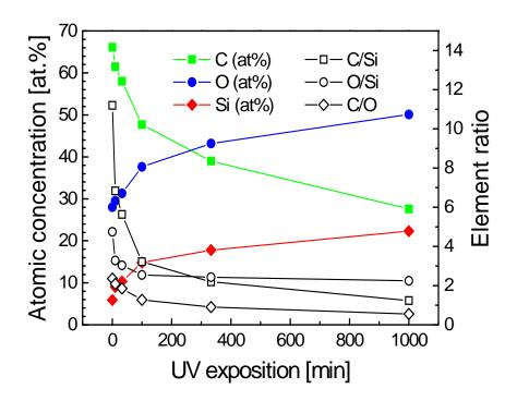
Figure 14: Elemental composition (carbon, oxygen, silicon) measured by XPS and element ratio of pp-TVS films as a function of UV exposition time.
