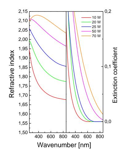
Figure 4: Dispersion curves for the refractive index and extinction coefficient of single layer films deposited at different RF powers
