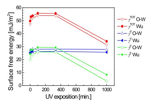
Figure 16: Dependence of the total surface free energy ( $\gamma^{TOT}$ ) and its component ( $\gamma^{d}$  – dispersion part,  $\gamma^{p}$  – polar part) evaluated according Owens-Wendt and Wu method on time of UV exposition
