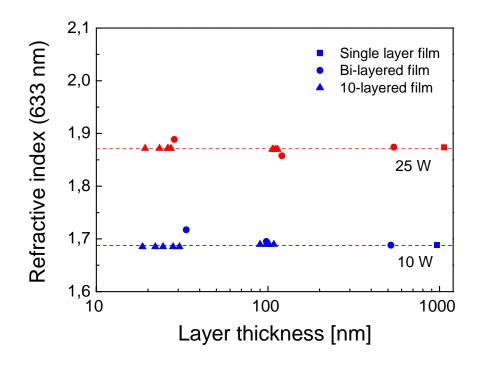
Figure 22: Refractive index at a wavelength of 633 nm as a function of layer thickness. Dashed line corresponding to the refractive index of single layer film is used as a guide for eye
