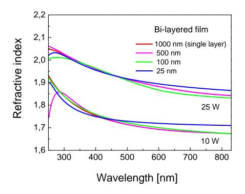
Figure 20: Dispersion curves for the refractive index of individual layers in bi-layered film. Dispersion curves corresponding to the individual layer of thickness 500, 100, and 25 nm are compared with that for single layer film
