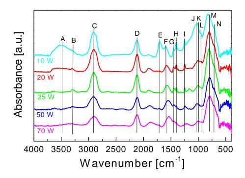
Figure 6: FTIR spectra of pp-TVS layers prepared at different RF powers
