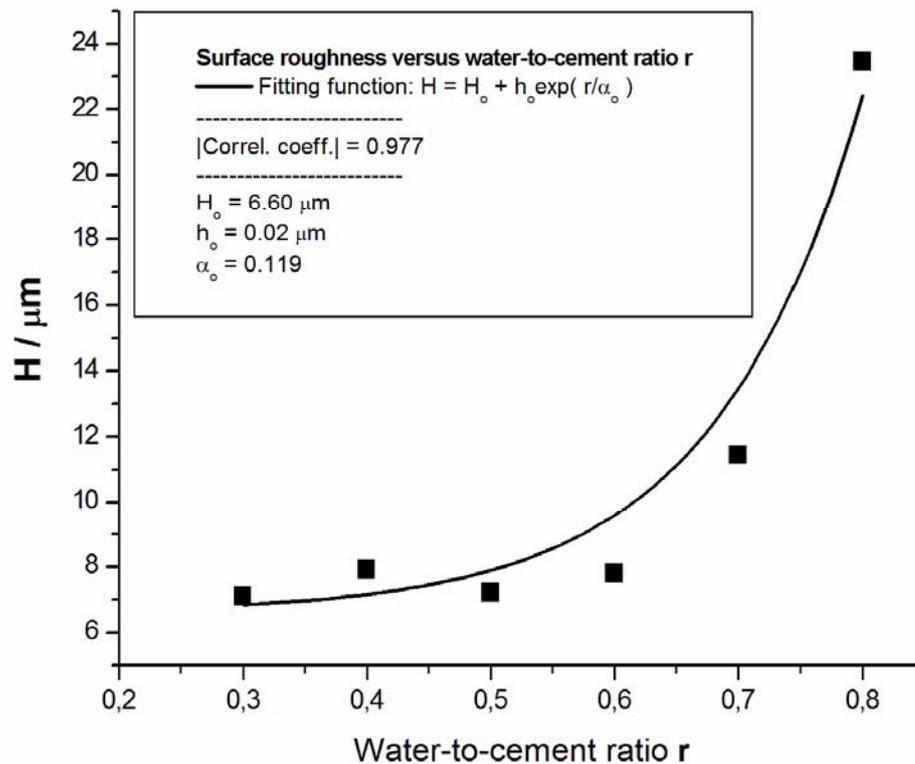
**Figure 2.** Surface irregularity  $H$  as a function of water-to-cement ratio  $r$
