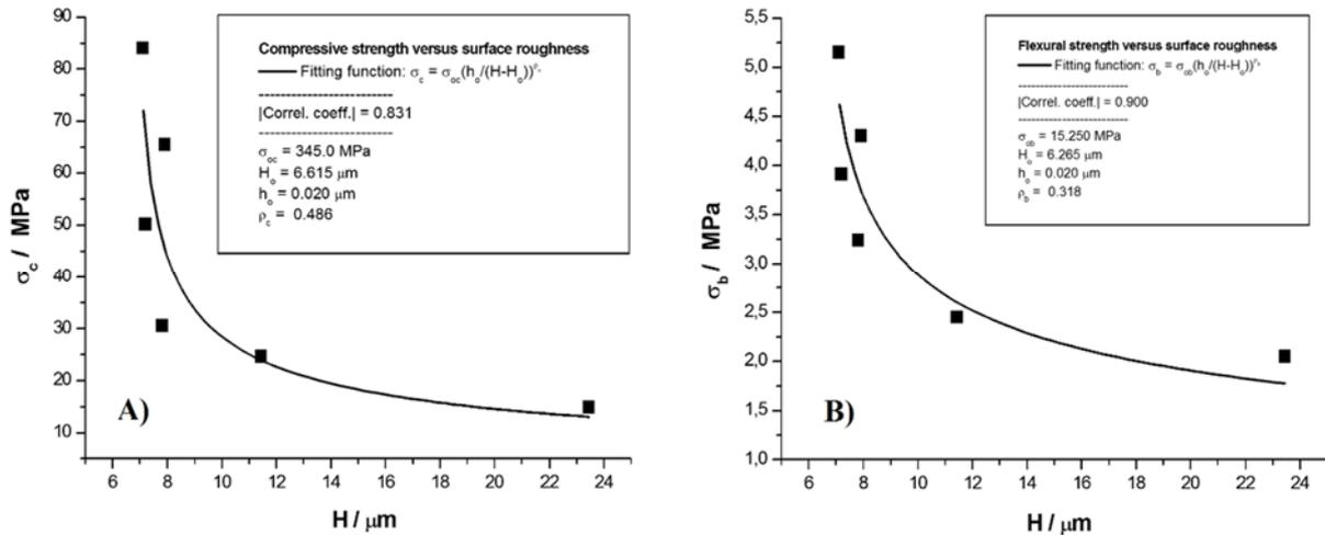
**Figure 3.** Mechanical strengths of hydrated Portland cement pastes as functions of surface irregularities quantified by the height parameter  $H$ : A) Compressive strength  $\sigma_c(H)$ ; B) Flexural strength  $\sigma_b(H)$ .
