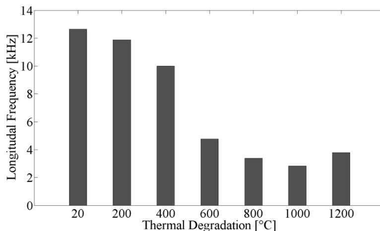
**Figure 4.** The change of dominant frequency of longitudinal waves versus the degree of thermal degradation.
