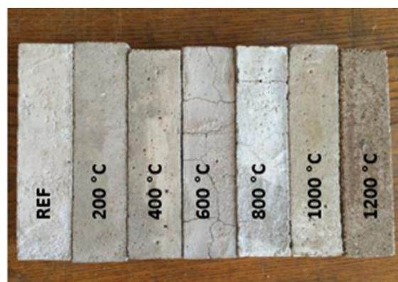
**Figure 3.** Specimens after thermal degradation.
