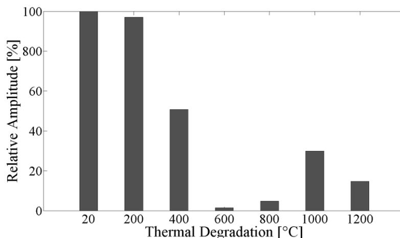
**Figure 6.** The change of relative amplitude versus the degree of thermal degradation.
