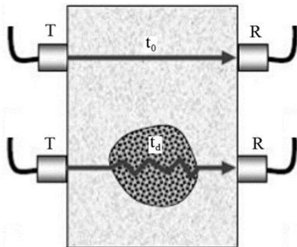
**Figure 2.** Principle of ultrasound measurement
