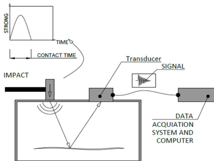
**Figure 1.** Principle of Impact-Echo measurement.
