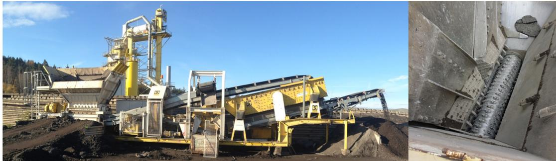
**Figure 2.** Reclaimed Asphalt Pavement granulator (left), a detail of the crushing chamber with the milling shaft (right), an asphalt plant with the fitted parallel drying drum in the background.
