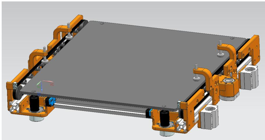
**Figure 2:** Automatic loading and leveling platform.
