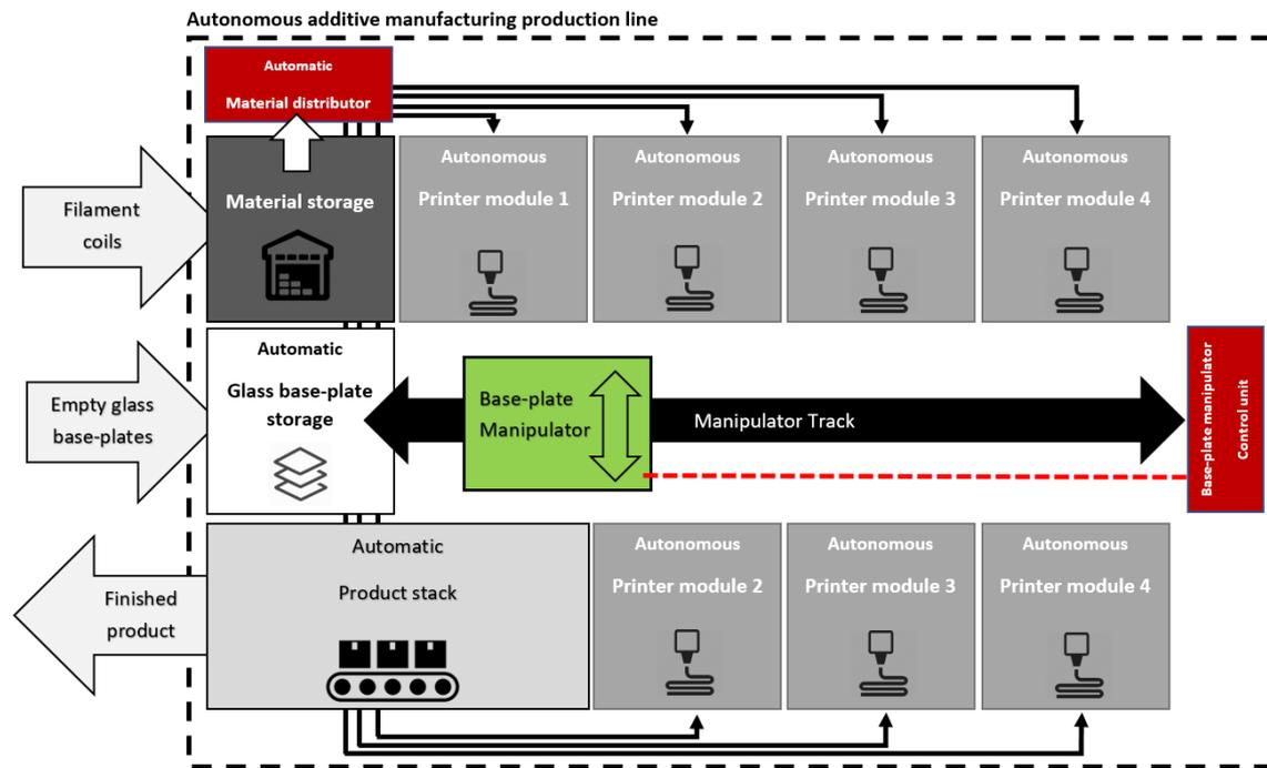
**Figure 1:** Topology of autonomous additive manufacturing production line.
