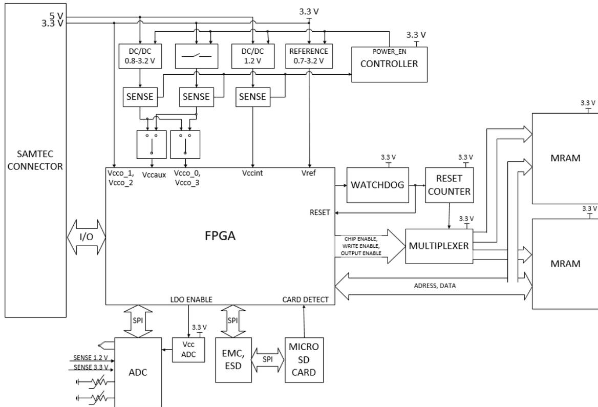
**Figure 1:** Block diagram of the control unit
