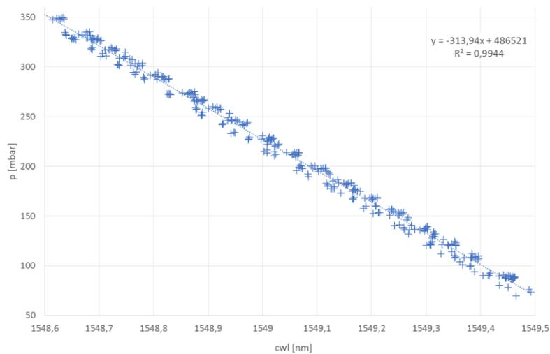
**Figure 4:** Calibration curve for optical pressure sensor
