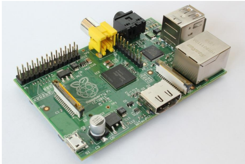
Obr. 2 Raspberry Pi model B [1].
