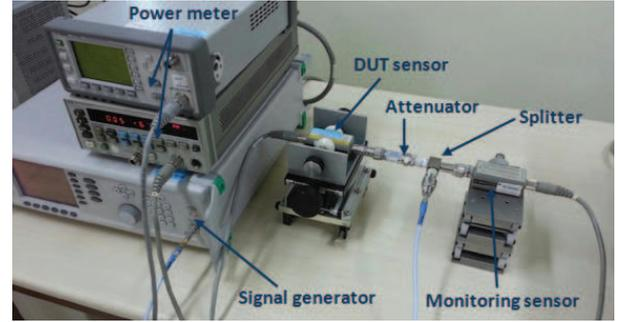
(a) The whole calibration system when the DUT sensor is connected to port 2 of the splitter through an attenuator
