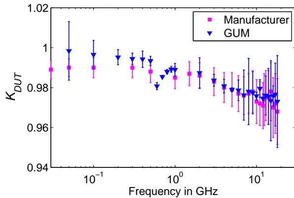
Fig. 7. The results provided by the manufacturer and estimated using the GUM (Uncertainty bars are shown for  $u_c$ ).
