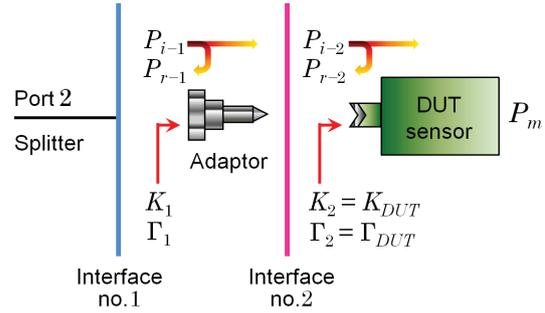
Fig. 2. Flow of the microwave power to a DUT power sensor with an adaptor.
