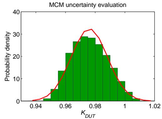
Fig. 5. Example of the simulated results using the Monte Carlo method with fitted distribution.
