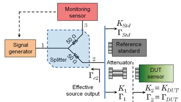
Fig. 1. Calibration of a high-sensitivity power sensor through an attenuator using direct comparison transfer technique.
