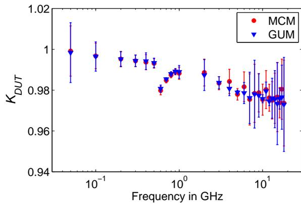
Fig. 6. The results estimated using the MCM and GUM methods (Uncertainty bars are shown for  $u_c$ ).
