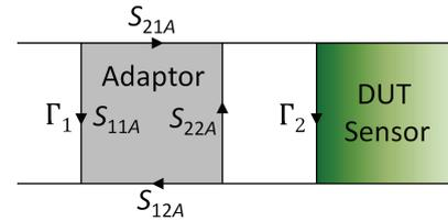
Fig. 3. A simplified flow-graph for an adaptor before a microwave power sensor corresponding to Fig. 2.
