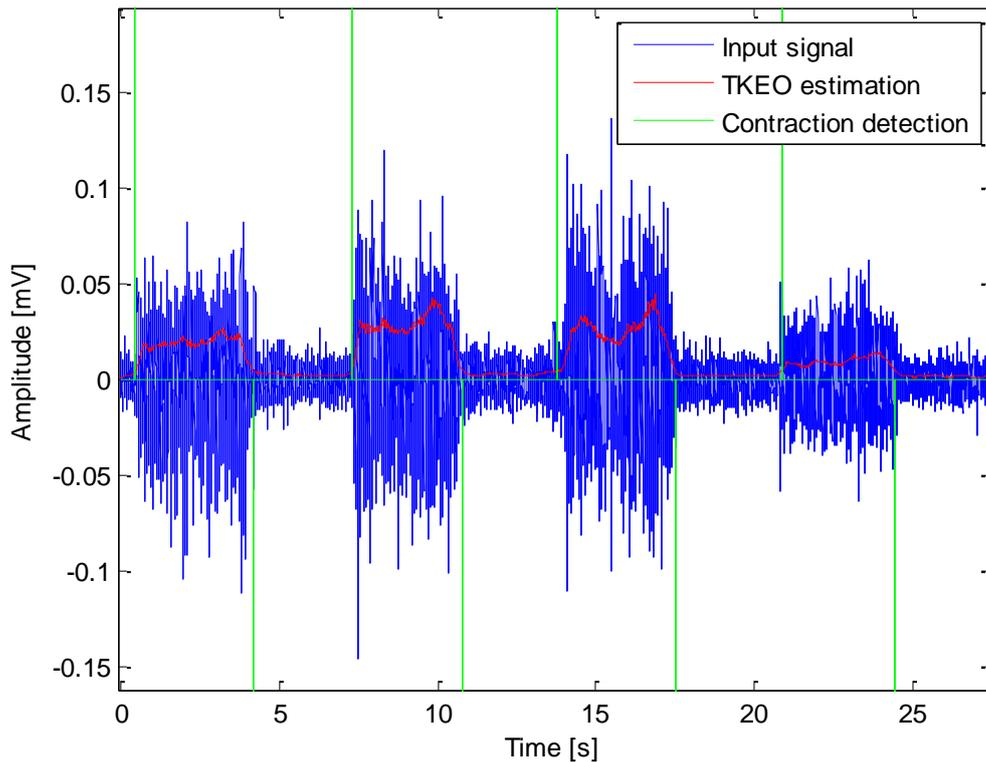
**Figure 1** - EMG signal before and after TKEO, with true positive onset and off-set detection
