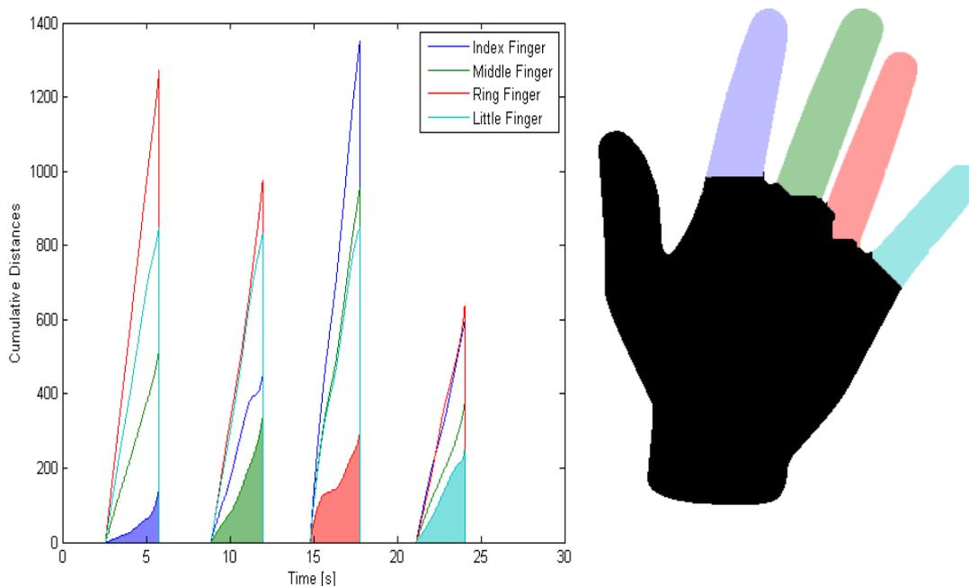
**Figure 3** - Output of the algorithm shows cumulative distances on the left and corresponding fingers
