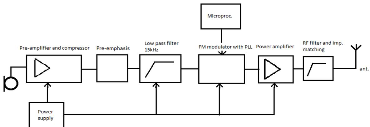
Figure 1: Block diagram
