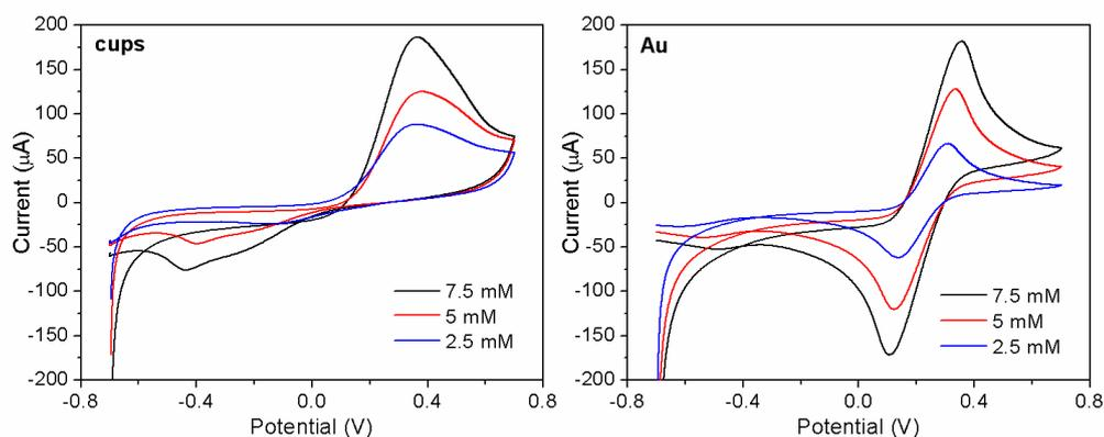
**Figure 5:** Cyclic voltammograms for various concentrations of potassium ferro-ferricyanide.
