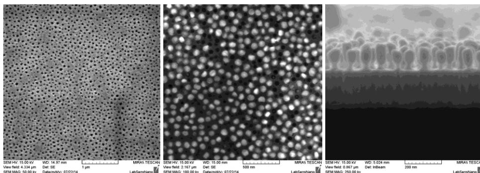
**Figure 2:** SEM images of alumina template (left), deposited gold into the nanoporous template (middle) and cross section of gold nanostructured surface (right).
