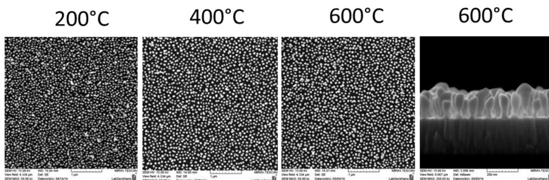
**Figure 4:** SEM images of samples annealed at various temperatures in vacuum (scale 1  $\mu\text{m}$ ) and cross section after 600°C vacuum annealing.
