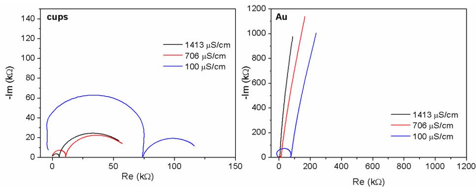
**Figure 6:** Nyquist plots of impedance spectra measured for nanostructured surface with cups and flat gold electrodes.
