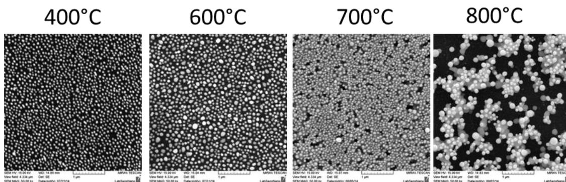
**Figure 3:** SEM images of samples annealed at various temperatures in air (scale 1  $\mu\text{m}$ ).
