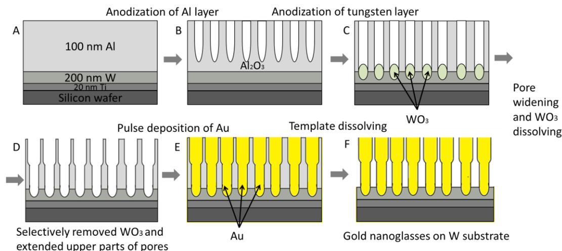
**Figure 1:** Scheme of production of gold nanostructured surfaces.
