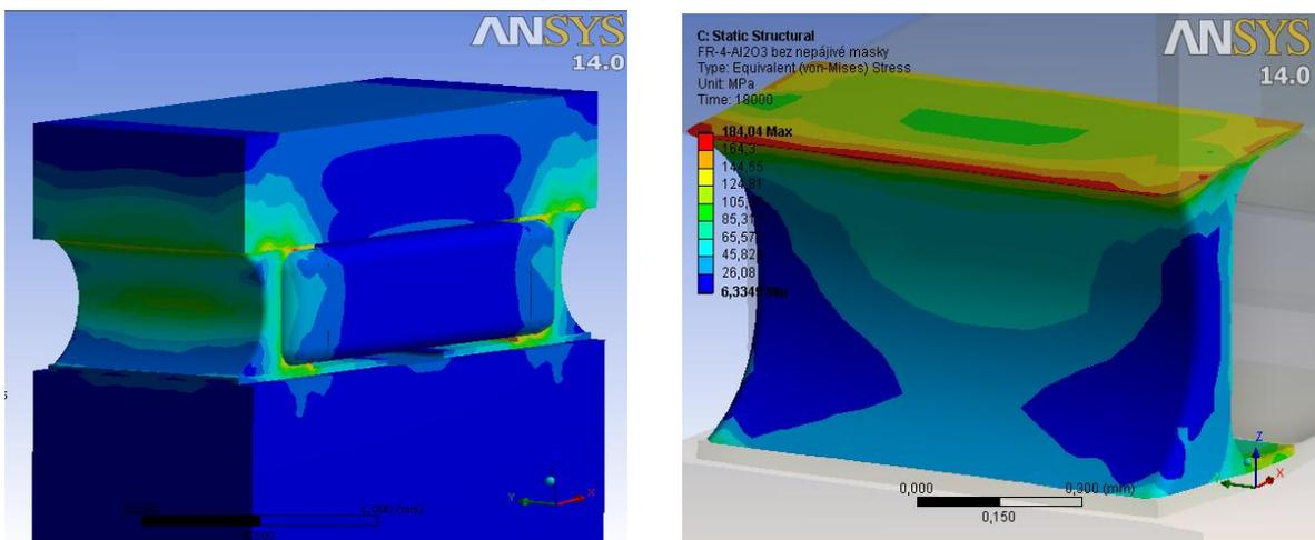
**Figure 3:** Von-Mises stress in ANSYS (a) Complete assembly (b) Detail of solder joint
