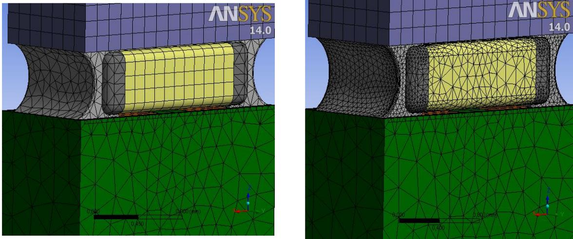
**Figure 2:** Mesh of nodes in ANSYS (a) Basic degree of mesh (b) Improved mesh
