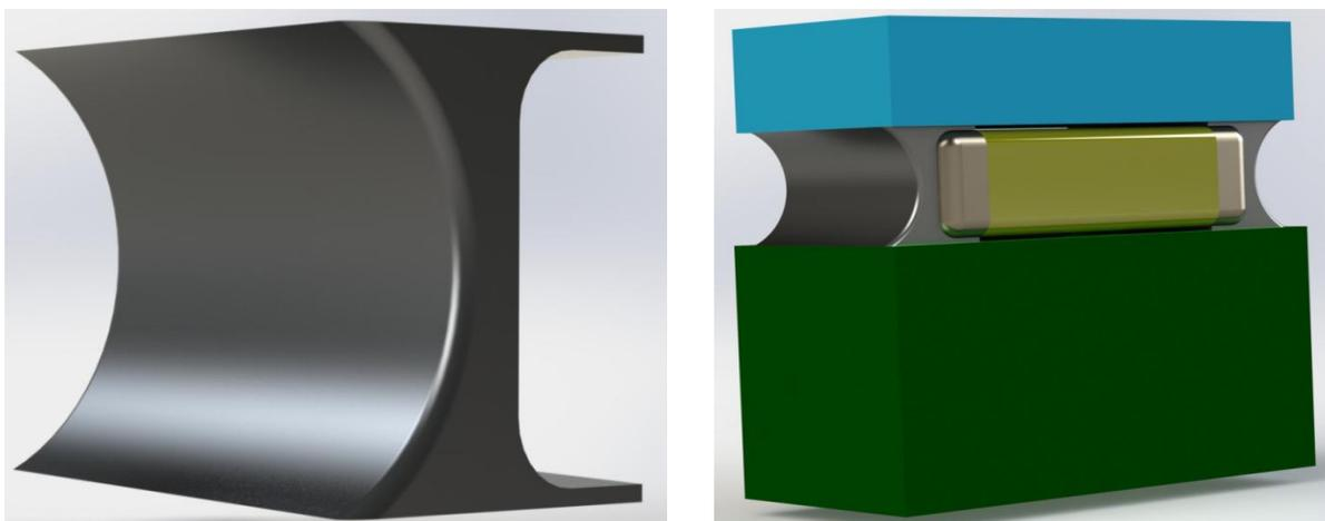
**Figure 1:** Models from Solidworks (a) Solder joint (b) Assembly FR-4-LTCC
