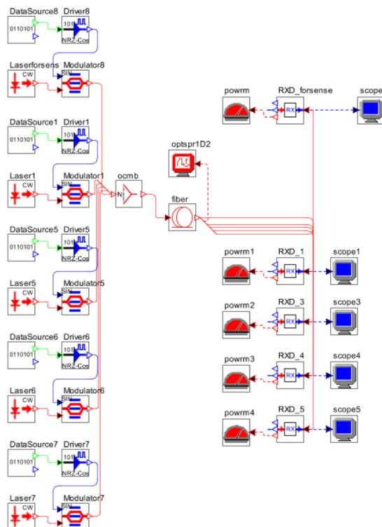
Figure 4.1: DWDM and Laser system configuration
