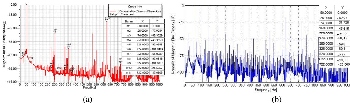
**Figure 2:** Spectrums of current (a) and magnetic flux density in the air-gap (b) of motor with 20% dynamic eccentricity.
