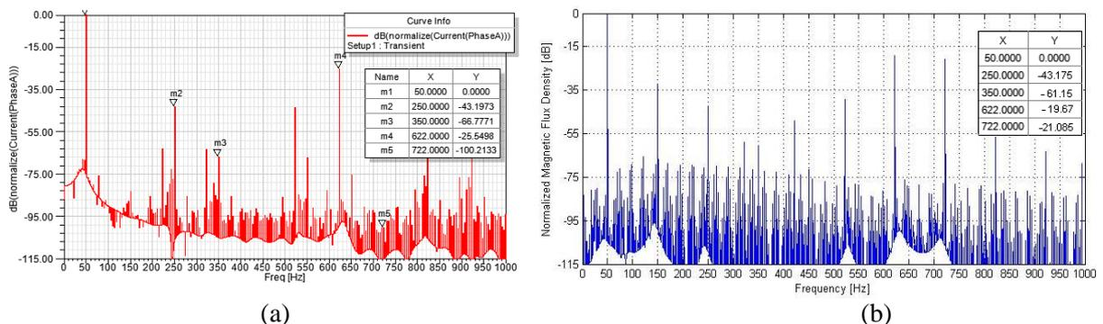
**Figure 1:** Current spectrum (a) and spectrum of magnetic flux density (b) of healthy motor.
