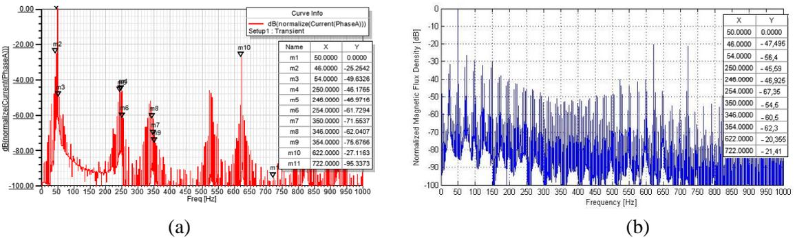
**Figure 4:** Spectrums of current (a) and magnetic flux density in the air-gap (b) of motor with broken rotor bars.
