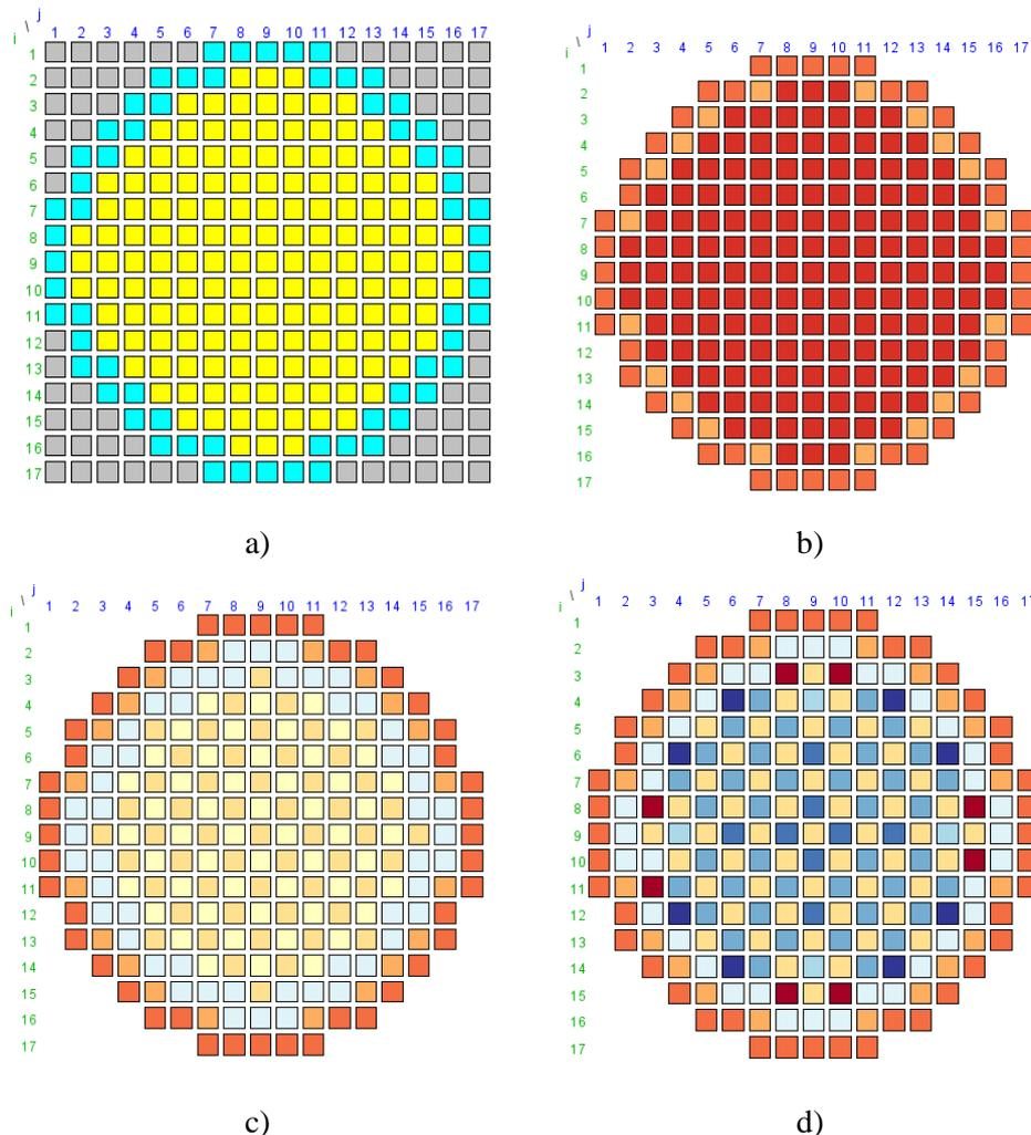
**Figure 1:** a) Core geometry (yellow – core, blue - reflector), b) Planar region at the top and bottom level, c) Planar region at 2nd level and d) core planar region
