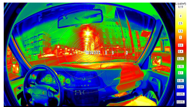
Fig.2. Picture for evaluation of distribution of luminance (Shutter time for HDR - 4 sec., 15 sec. and 30 sec.)
