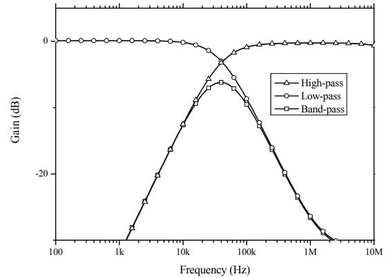
Fig. 16. Gain responses of the filter given in Fig. 7.
