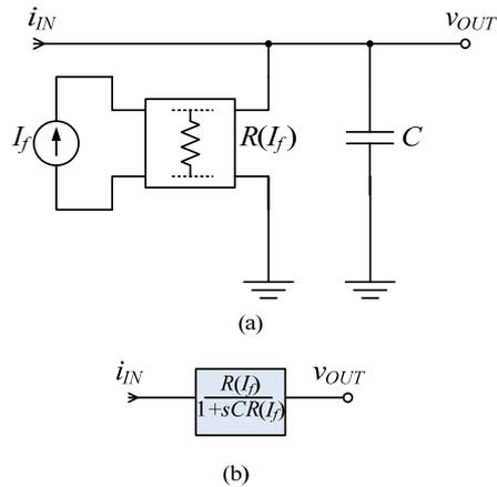
Fig. 4. (a) Electronically tunable lossy integrator circuit and (b) its block.
