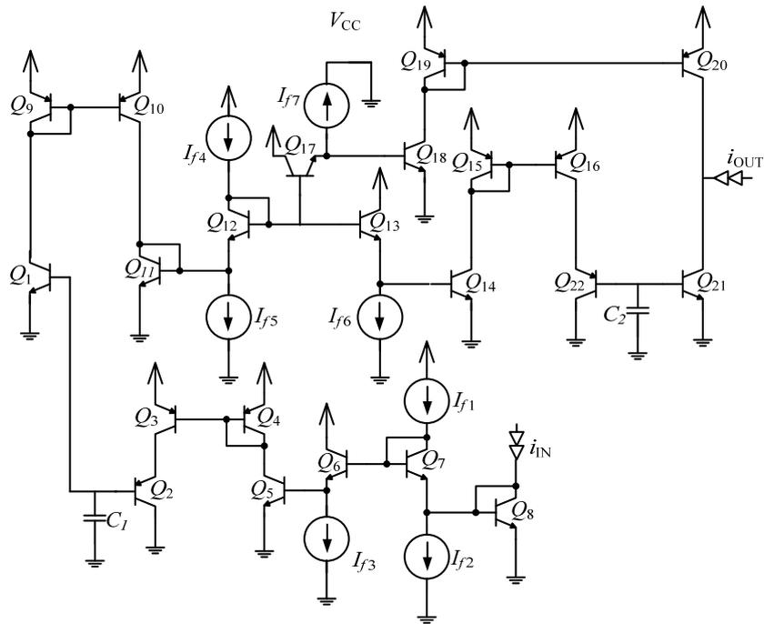
Fig. 7. Complete circuit of the second-order band-pass filter.
