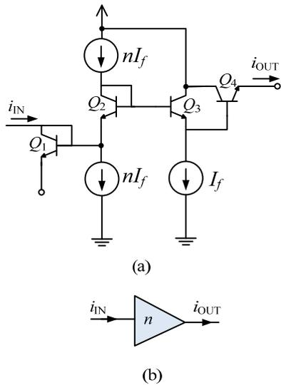
Fig. 3. (a) Constant multiplying circuit and (b) its block.
