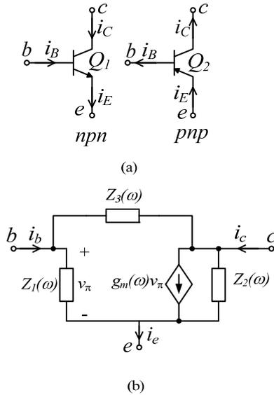
Fig. 1. (a) Electrical symbols of both of *npn*-type and *pnp*-type BJTs and (b) their small signal model.
