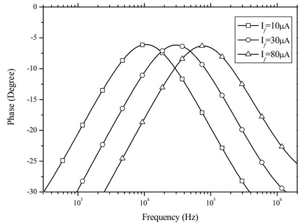
Fig. 17. Gain responses of the second-order band-pass filter against frequency for various control currents  $I_f$ .
